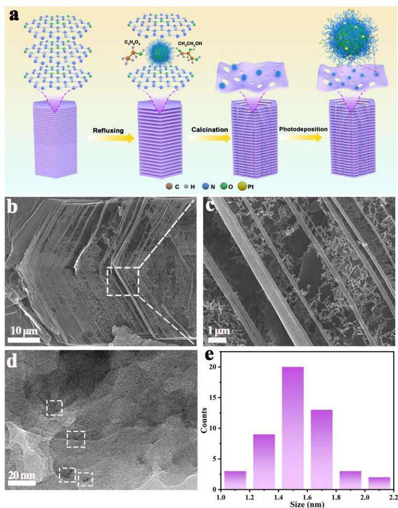
**Figure 1.** (a) Schematic illustration of the preparation process of Pt-CDs/ $C_3N_4$ , (b,c) SEM images of CDs/ $C_3N_4$ , (d) HR-TEM images of CDs/ $C_3N_4$  (The white boxes highlight the loaded CDs), and (e) the particle size distribution map of CD nanoparticles on  $C_3N_4$ .
