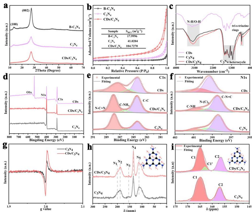
**Figure 2.** (a) XRD patterns of  $CDs/C_3N_4$ ,  $C_3N_4$ ,  $B-C_3N_4$ . (b) Nitrogen adsorption desorption isotherms of  $CDs/C_3N_4$ ,  $C_3N_4$ ,  $B-C_3N_4$ ; (c) FT-IR spectra of  $CDs$ ,  $CDs/C_3N_4$ , and  $C_3N_4$ ; (d) XPS survey spectrum of  $CDs$ ,  $C_3N_4$ , and  $CDs/C_3N_4$ . (e)  $C1s$  and (f)  $N1s$  XPS spectra of  $CDs$ ,  $CDs/C_3N_4$ , and  $C_3N_4$ . (g) EPR spectra, (h)  $^{15}N$  and (i)  $^{13}C$  NMR spectra of  $C_3N_4$  and  $CDs/C_3N_4$ .
