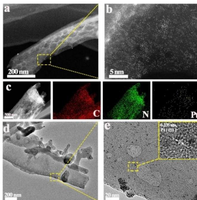
**Figure 4.** (a,b) Representative HAADF-STEM image of Pt-CDs/C<sub>3</sub>N<sub>4</sub>; (c) the corresponding EDX maps of Pt-CDs/C<sub>3</sub>N<sub>4</sub>. (d,e) TEM and HRTEM image of the Pt-C<sub>3</sub>N<sub>4</sub>.
