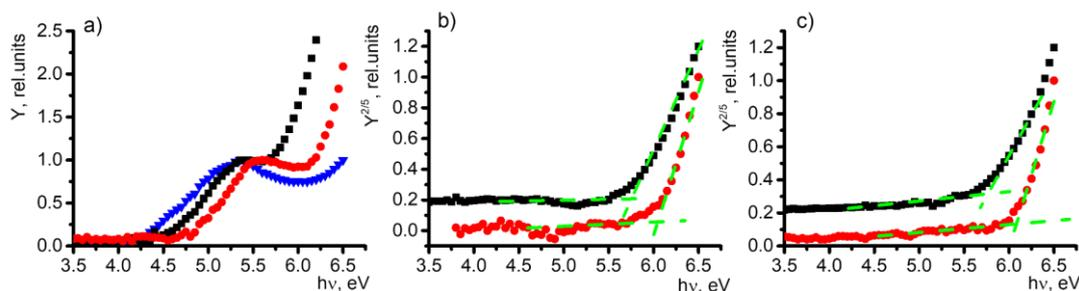
**Figure 1.** Photoelectron emission yield spectra of 2PACz (black squares), Cl-2PACz (red circles), and ITO (blue triangle) in (a) SAM films, (b) SAM films without ITO signal, and (c) bulky samples. Cross point of green lines represents the obtained energy.
