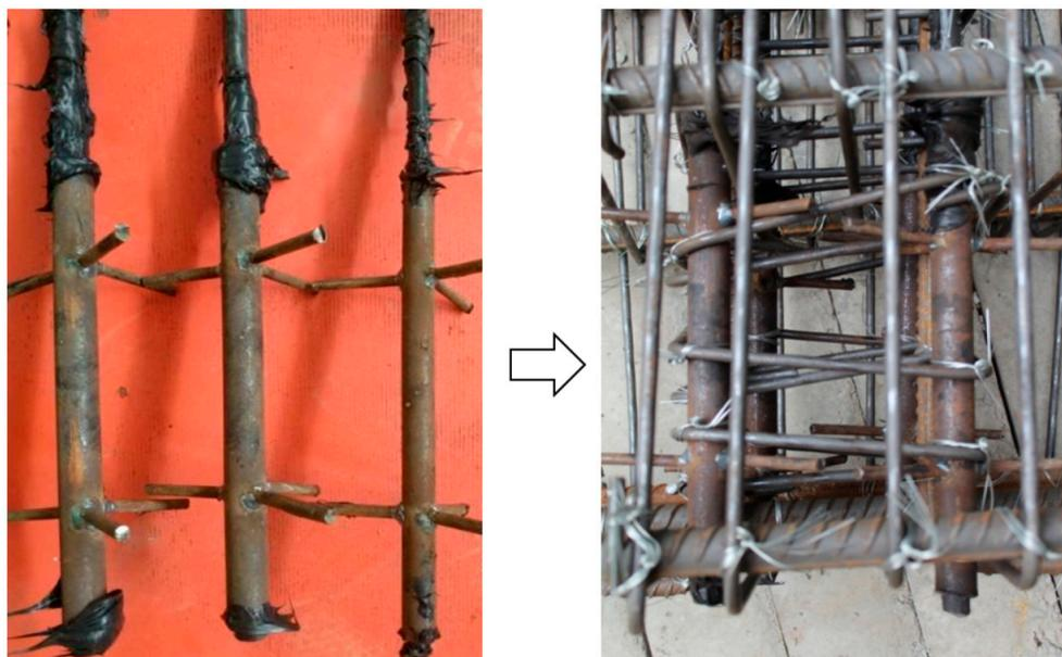
Figure 3. End anchoring of FRP bars.
