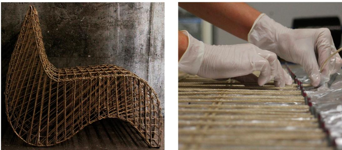
**Figure 8.** The hemp chair during production, with an emphasis on the winding process applied for the lignocellulosic endless fibres that are pre-soaked in the resin bath. Photo credit: Sachin and Kauffmann, BioMat-ITKE/University of Stuttgart.
