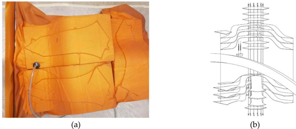
**Figure 3.** (a) Vacuum-pressing fabrication technique applied in the production of the sandwich panels using the closed molding technique; (b) Isometric view of single layers and connections of one of the four details of the applied modular system. © BioMat/ITKE-University of Stuttgart.
