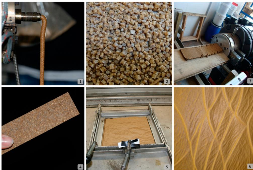
**Figure 1.** Up: (1) Compounding, (2) pelletising, and (3) extrusion processes. Down: (4) Cut panel, (5) the thermoforming-process of a thermoplastic biocomposite panel, and (6) a thermoformed final finished panel (photos: Dahy, H.; republished [8]).
