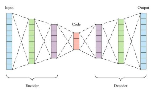
Figure 1. A general autoencoder architecture.
