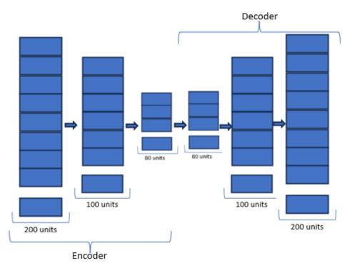
Figure 2. Encoder-decoder based novel LSTM and GRU architectures.
