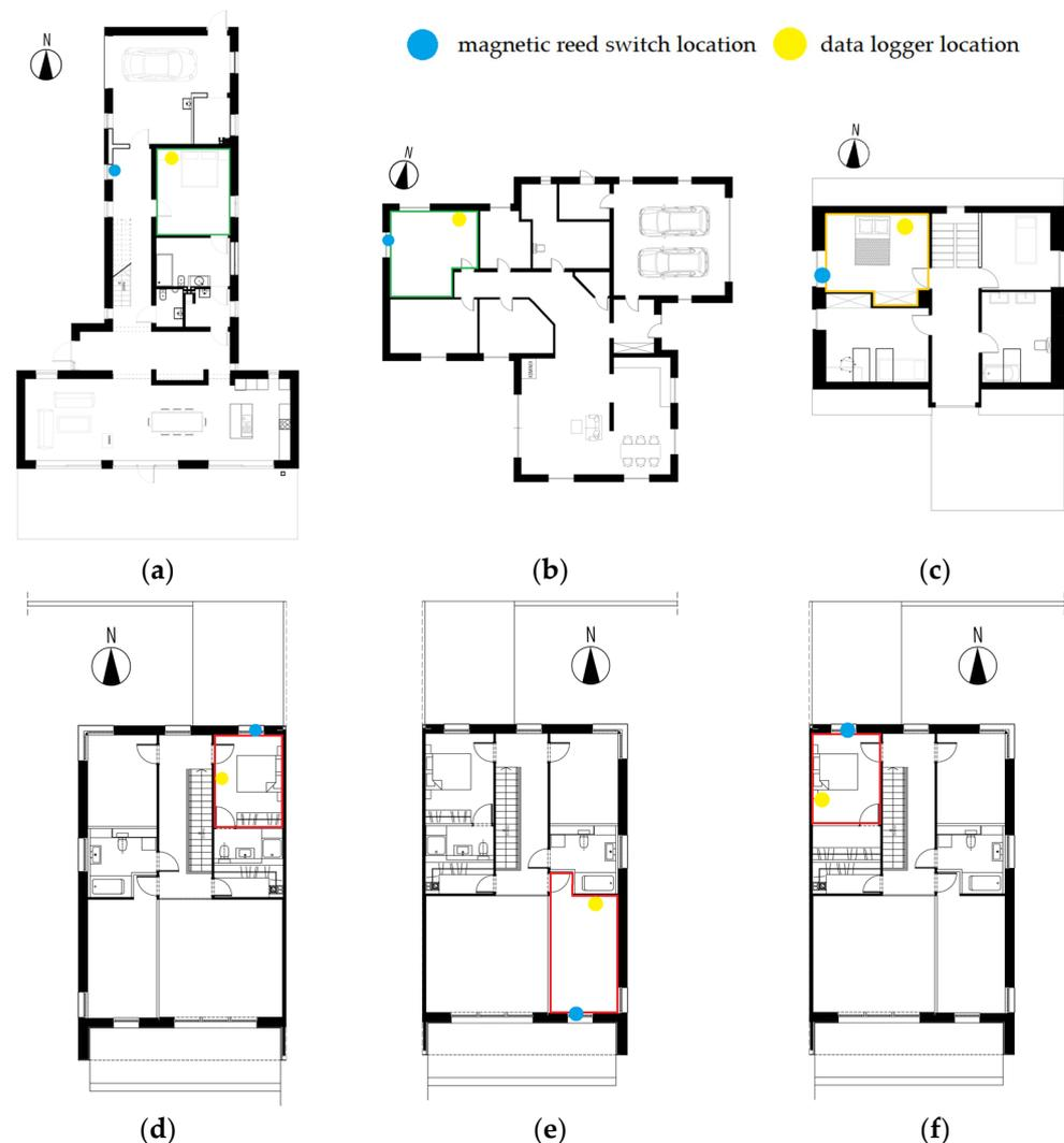
**Figure 1.** Location of measuring equipment: (a) NV1; (b) NV2; (c) HV1; (d) MV1; (e) MV2; (f) MV3.
