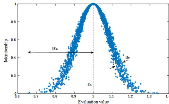
**Figure 3.** One-dimensional cloud model.
