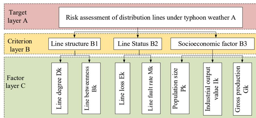
**Figure 1.** Risk assessment index system of distribution network in typhoon weather.
