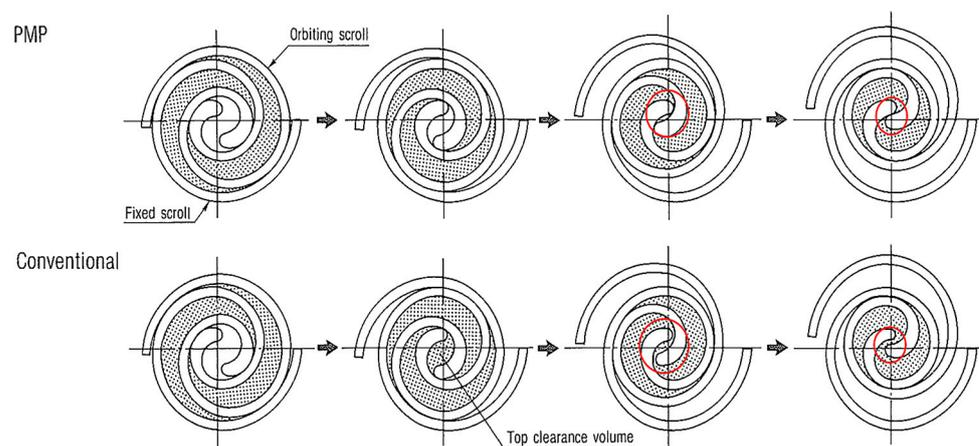
**Figure 4.** Characteristics of PMP and conventional profile described by Takahisa [34].
