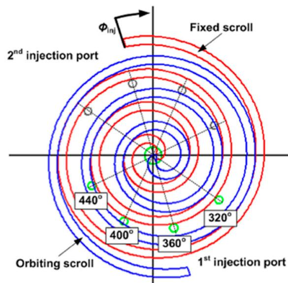
Figure 10. Two different injection ports [72].
