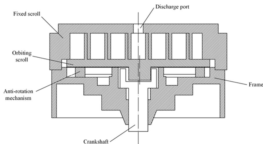
**Figure 2.** Structure of scroll compressor by Yu [15].
