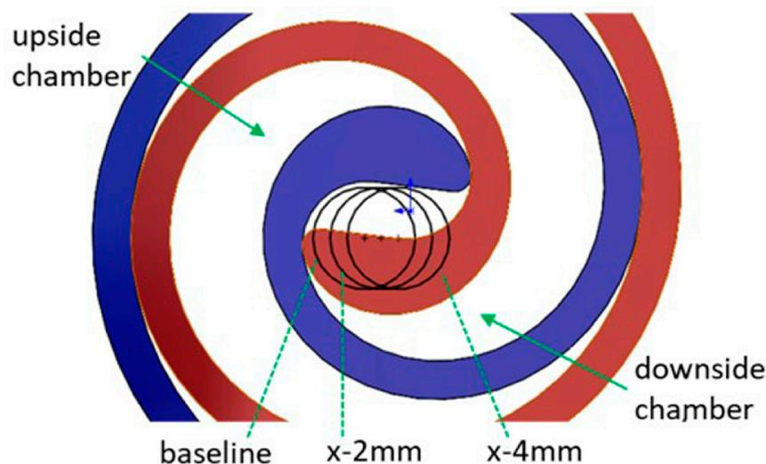
**Figure 5.** Three different discharge ports as described by Zhao [52].
