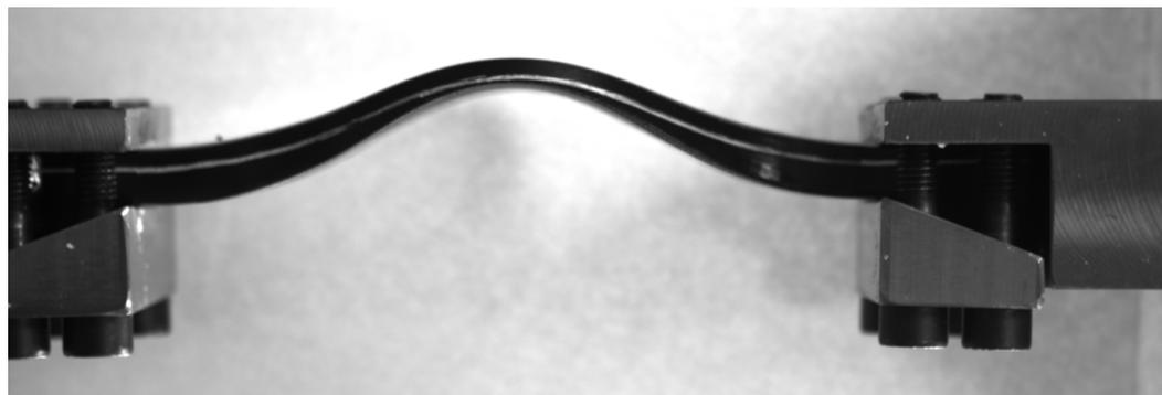
**Figure A2.** Buckling of the hinge during compression test.
