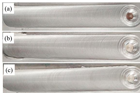
**Figure 4.** The weld surfaces of the friction stir welds (FSWs) under different states: (a) T1; (b) T4; (c) T6.
