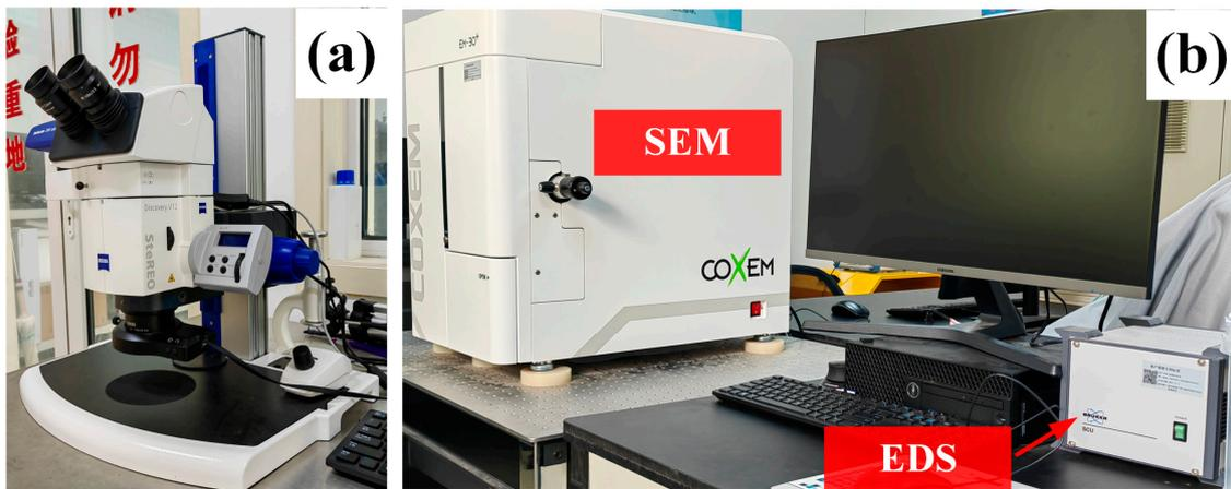
**Figure 4.** Fracture analysis system: (a) optical microscope (OM); (b) scanning electron microscope (SEM) and energy dispersive spectrometer (EDS).
