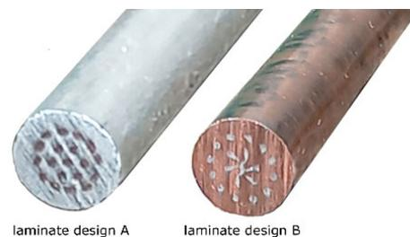
**Figure 2.** Final 5 mm swaged laminates of design A (Al sheath), and design B (Cu sheath).
