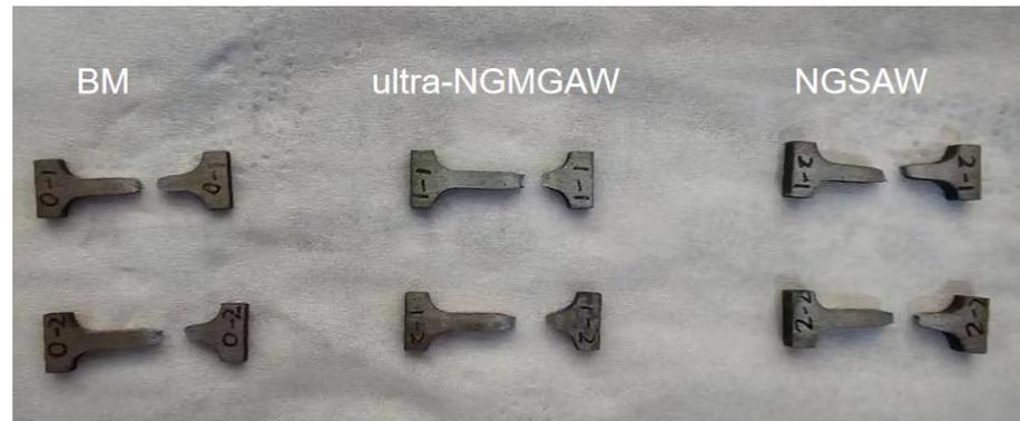
Figure 10. Tensile specimen after fracture.
