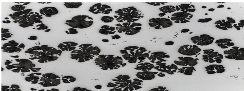
**Figure 1.** Examples of images of cast iron microstructures used in the research.
