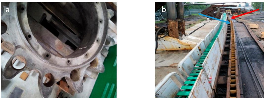
**Figure 14.** Elements of the longwall shearer haulage system: (a) drive wheel; (b) track.
