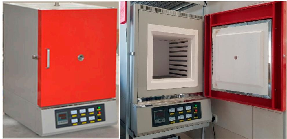
**Figure 4.** KJ-M1200-64L-IC muffle furnace used in the experiment to heat the tested samples in the simulation of a fire incident.
