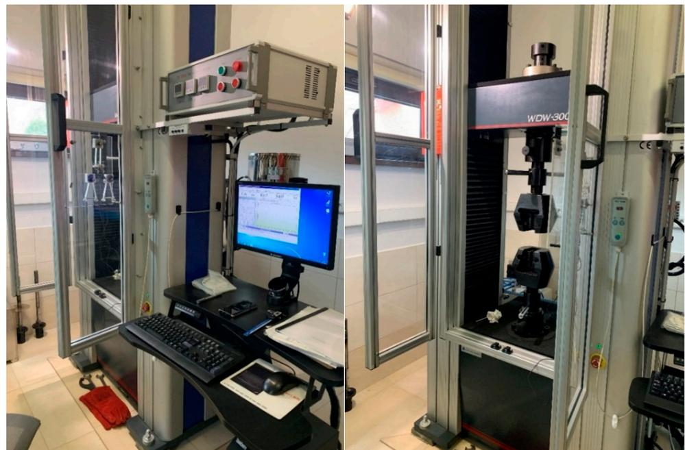
**Figure 1.** Testing setup for the static tension testing of samples cooled after surviving a simulated fire incident.
