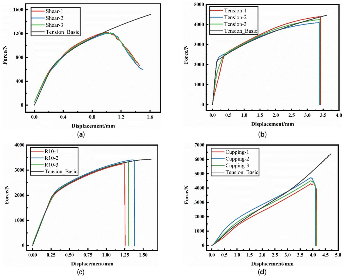
**Figure 3.** The loading–displacement curves of specimens under different stress states were tested: (a) shear test; (b) unidirectional tensile test; (c) R10 notch tensile test; (d) cupping test.
