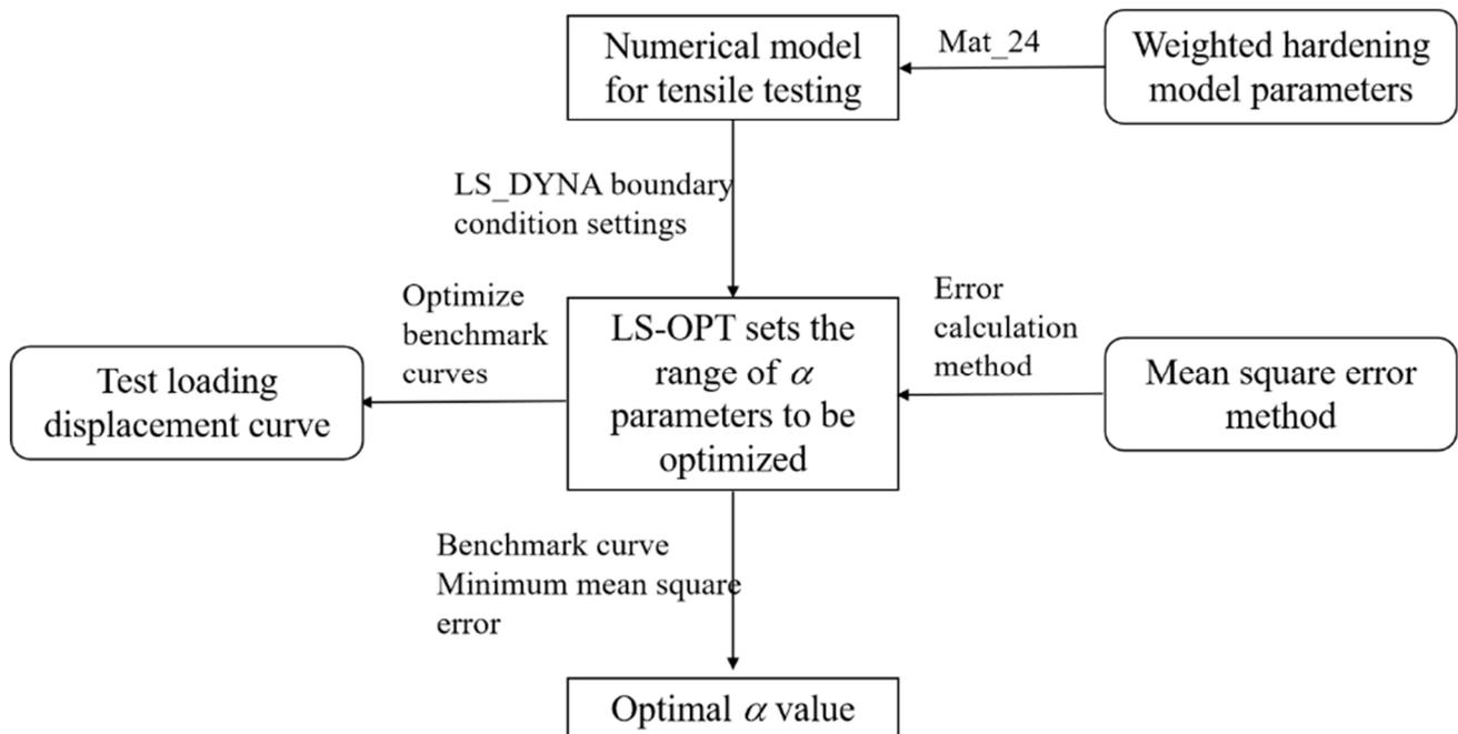
**Figure 6.** Parametric inverse process of weighted coefficient  $\alpha$  under uniaxial stress state.
