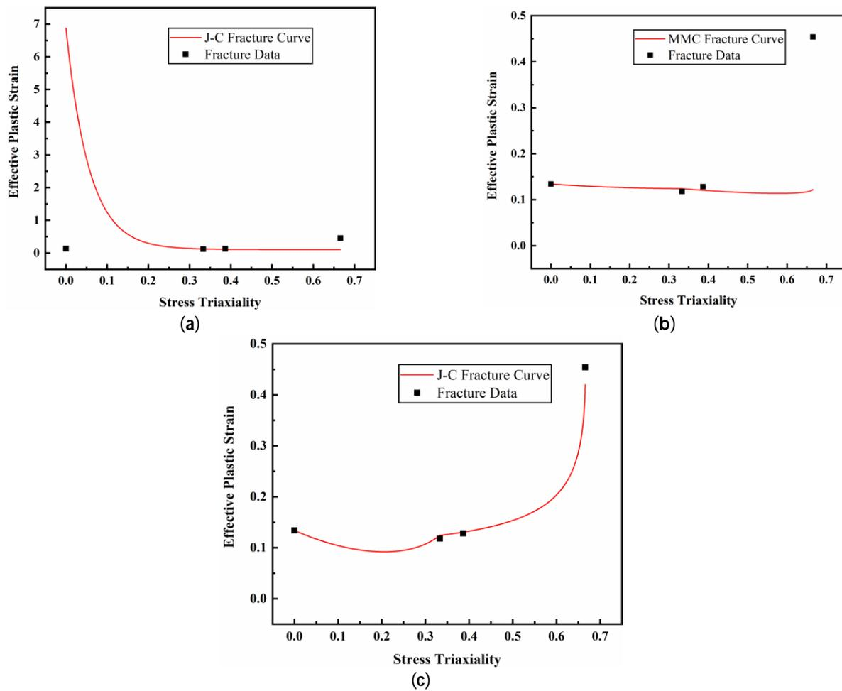
**Figure 14.** Each fracture model fits the curve: (a) JC fracture model curve; (b) MMC fracture model curve; (c) DIEM fracture model curve.
