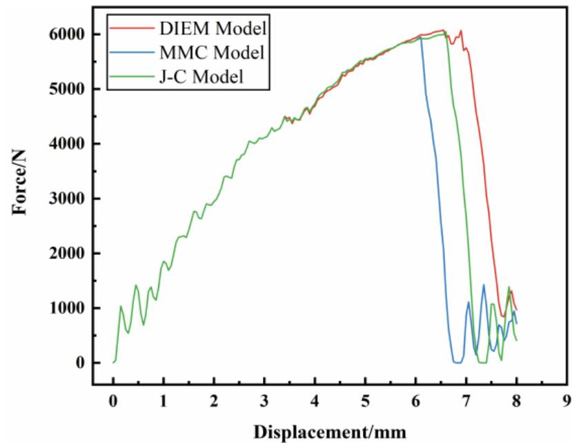
**Figure 17.** Three-point static simulation loading–displacement curve of front-end component.
