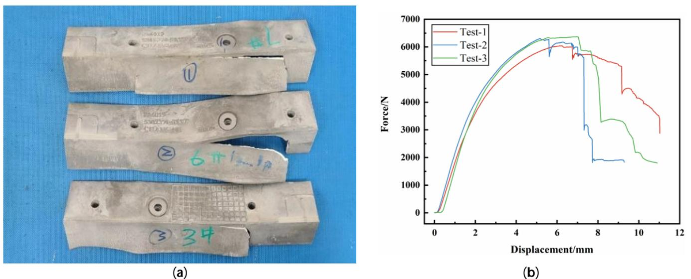
**Figure 19.** Three point static pressure test results of front-end components: (a) fracture shape of front end member; (b) loading–displacement curve.
