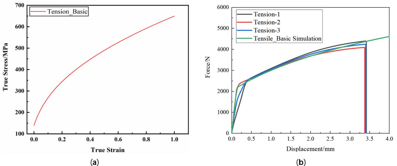
**Figure 7.** Inverse results of LS OPT parameters of uniaxial stress state constitutive model: (a) epitaxial true stress–plastic strain curve; (b) benchmarking results of loading–displacement curves.
