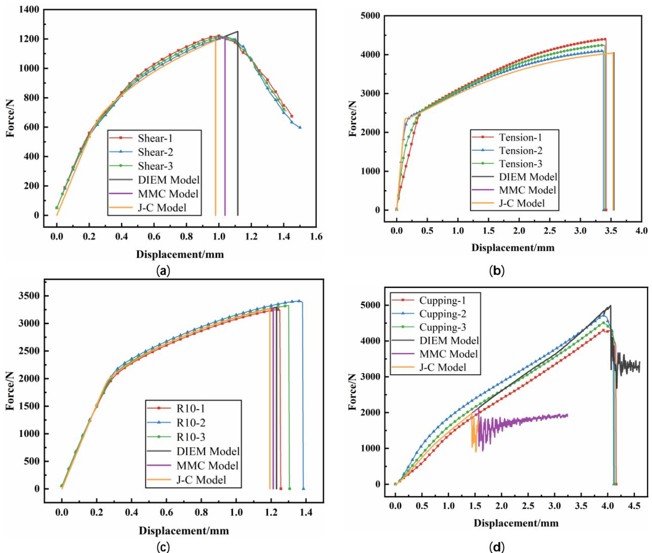
**Figure 15.** Three kinds of fracture predict the loading–displacement curves of specimens under different stress states: (a) shear test; (b) unidirectional tensile test; (c) R10 tensile test; (d) cupping test.
