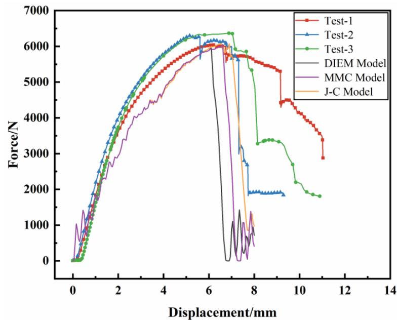
**Figure 20.** Comparison of three-point static pressure simulation of front-end component with experimental loading–displacement curve.
