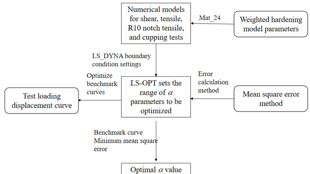
**Figure 9.** Inverse flow of parameters of weighted coefficient  $\alpha$  under complex stress state.
