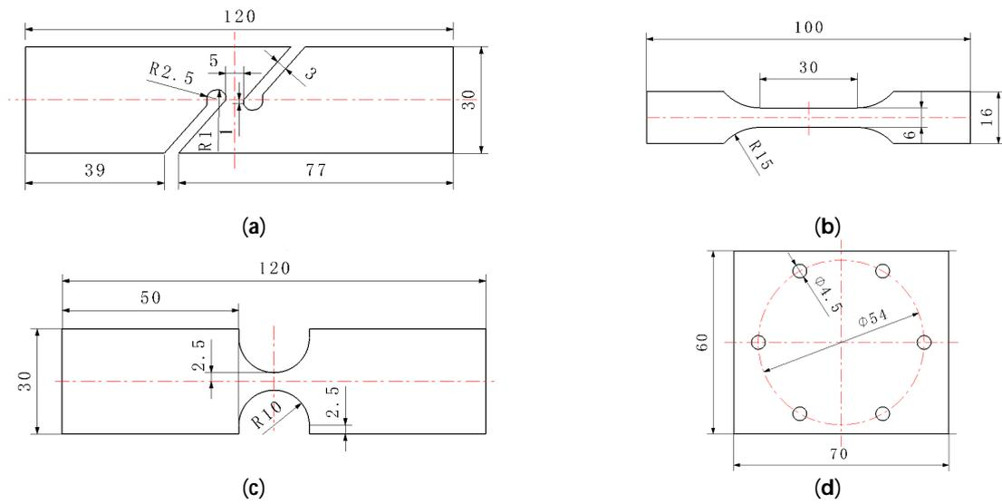
**Figure 2.** Sample size of the AM60B die-cast magnesium alloy sheet under different stress states (mm), (a) shear specimen; (b) unidirectional tensile specimen; (c) R10 notch tensile specimen; (d) cup specimen.
