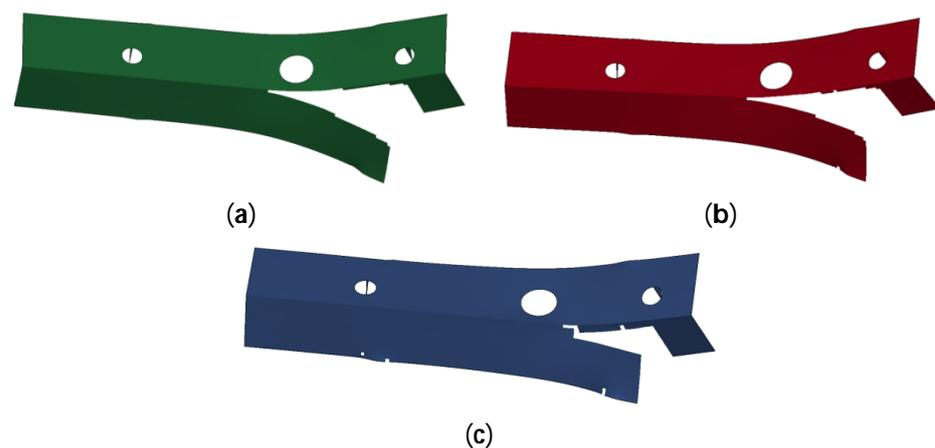
**Figure 18.** Three-point static simulation of fracture shape of front-end component: (a) JC model simulation result; (b) MMC model simulation result; (c) DIEM model simulation result.
