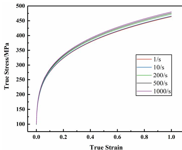
Figure 13. Dynamic constitutive relationship curve of the AM60B die-cast magnesium alloy sheet.
