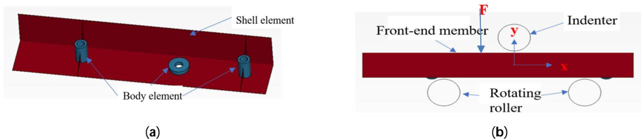
**Figure 16.** The three-point static simulation model of front-end component is established: (a) front-end component model; (b) three-point static simulation model.
