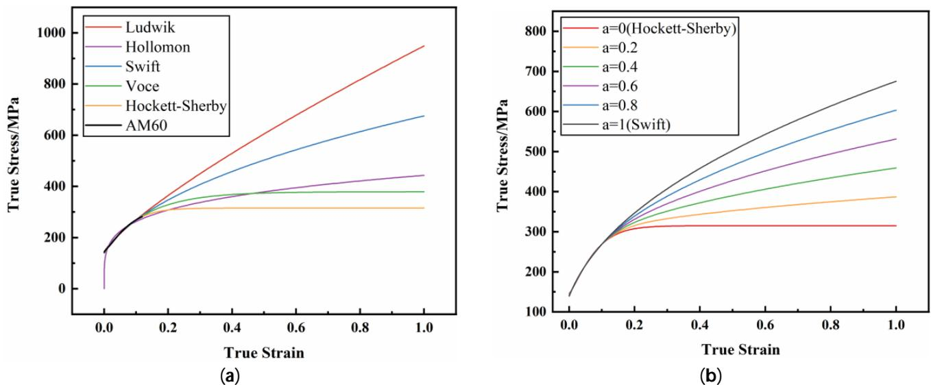
**Figure 5.** The true stress–plastic strain curve hardening model fits epitaxy: (a) different hardening models fit epitaxy; (b) fitting epitaxy with different weighting coefficients.
