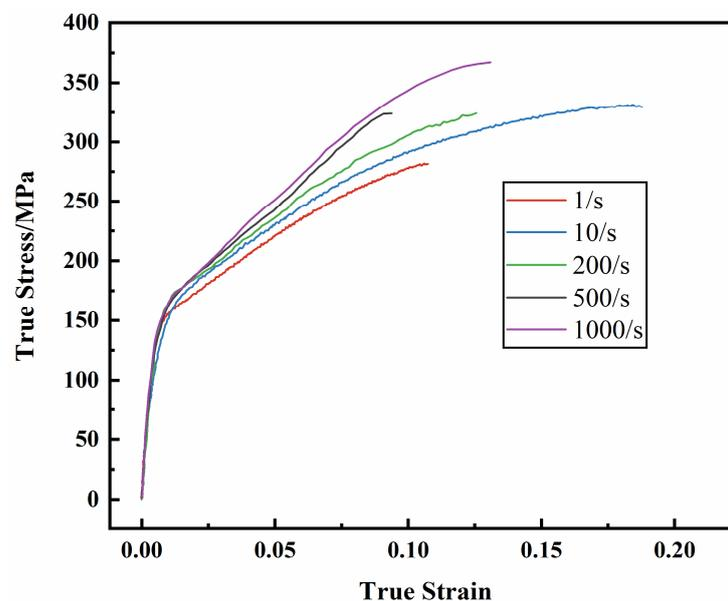
**Figure 12.** True stress–strain curves under different strain rates.
