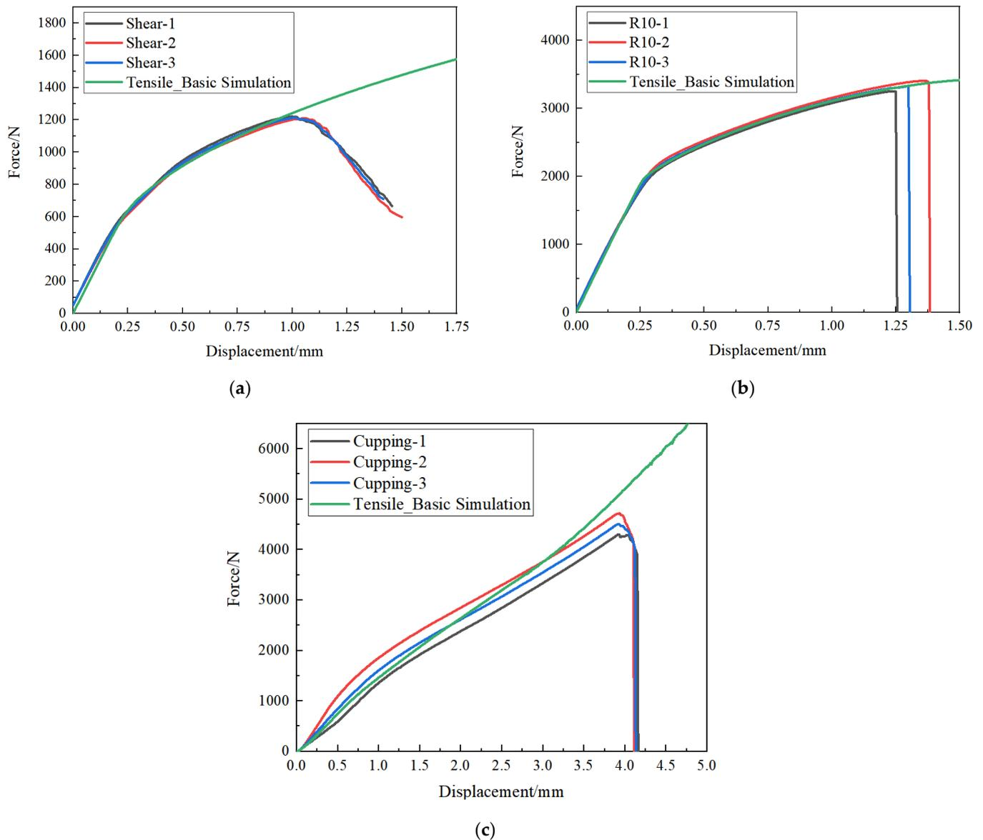
**Figure 8.** The benchmarking results of loading–displacement curves of tests under different stress states: (a) shear test; (b) R10 notch tensile test; (c) cupping test.
