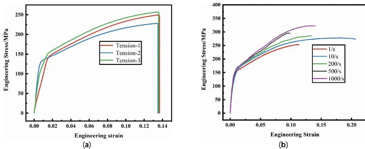
**Figure 1.** Engineering stress–engineering strain curve of the AM60B die-cast magnesium alloy sheet: (a) quasi-static tension; (b) dynamic tension.
