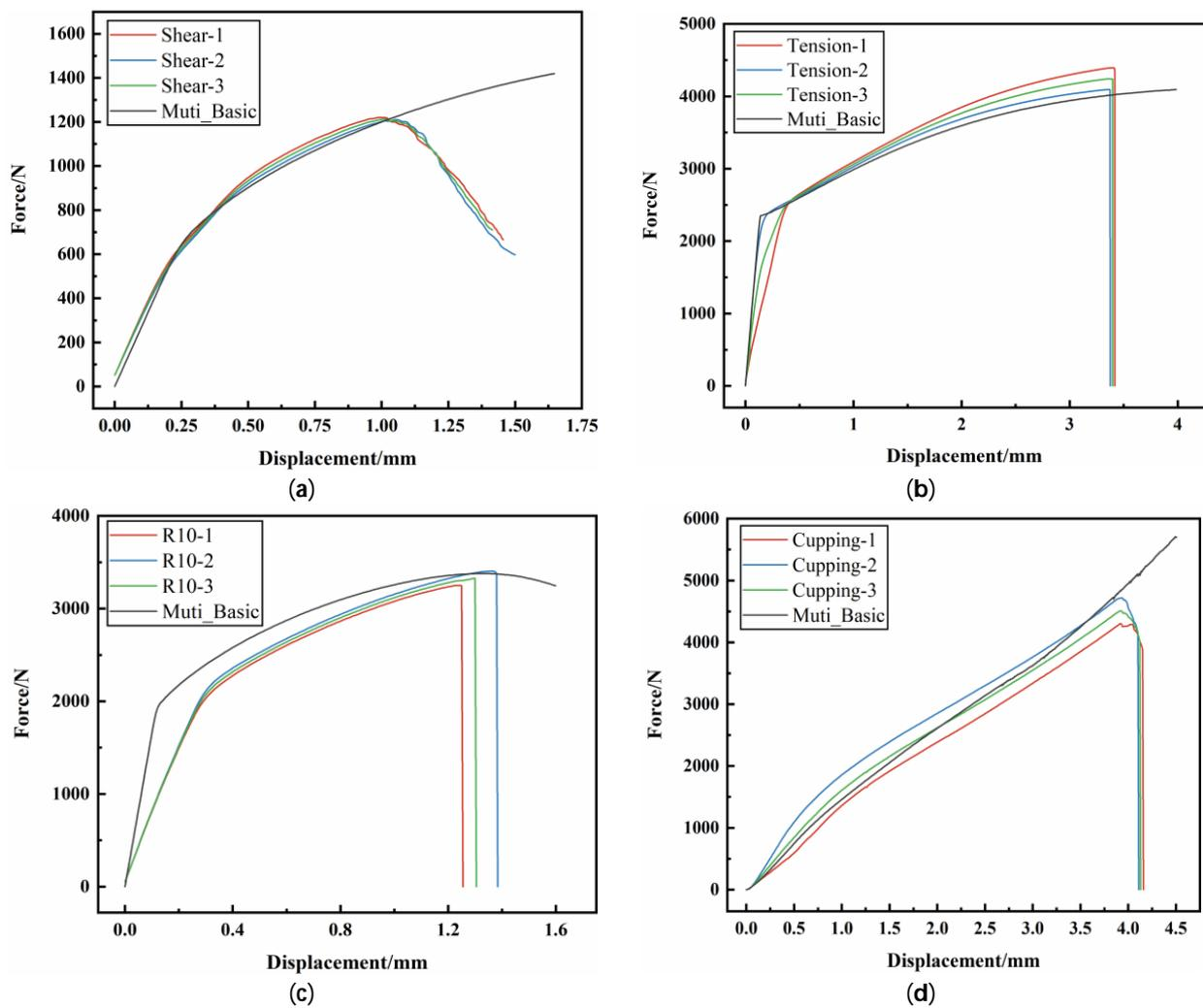
Figure 11. The benchmarking results of loading–displacement curves of each sample: (a) shear test; (b) unidirectional tensile test; (c) R10 notch tensile test; (d) cupping test.
