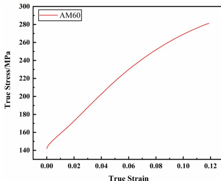
Figure 4. Quasi-static true stress–plastic strain curve of the AM60B die-cast magnesium alloy.
