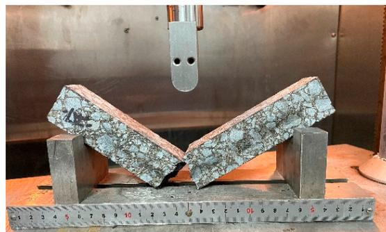
**Figure 4.** Illustration of trabecular bending test.
