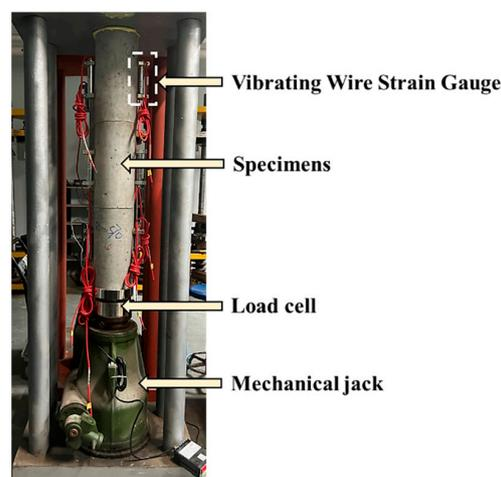
**Figure 4.** Creep test device.
