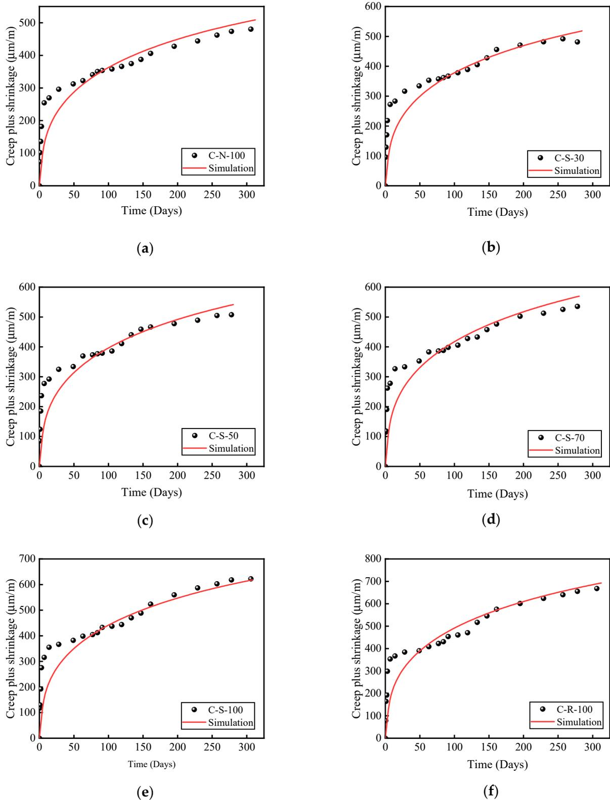
**Figure 10.** Comparison of experimental and simulated curves. (a) C-N-100. (b) C-S-30. (c) C-S-50. (d) C-S-70. (e) C-S-100. (f) C-R-100.
