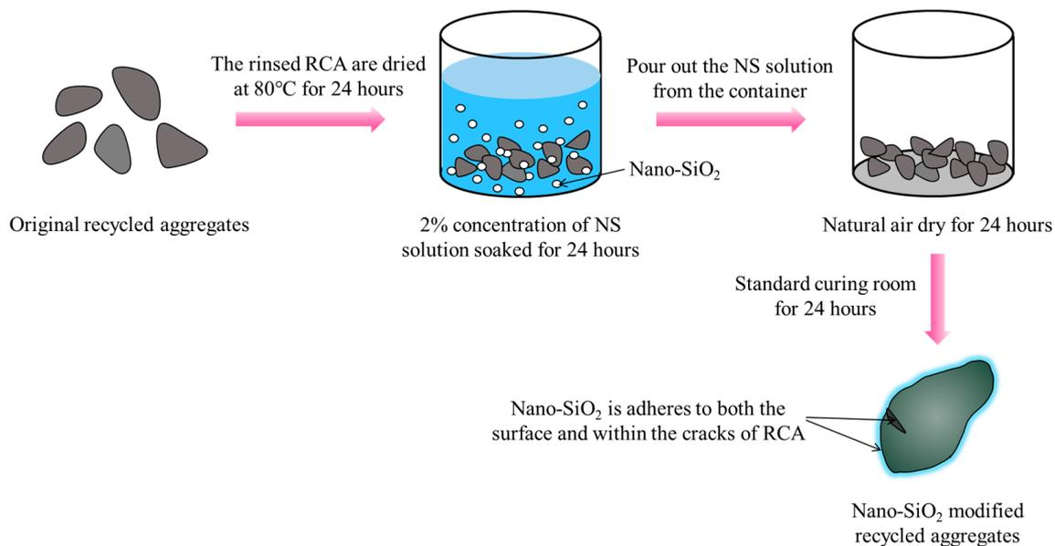
**Figure 3.** The modification process of RCA.
