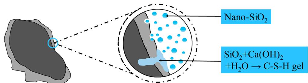
**Figure 1.** Strengthening mechanism of nano- $\text{SiO}_2$ -modified recycled aggregate.
