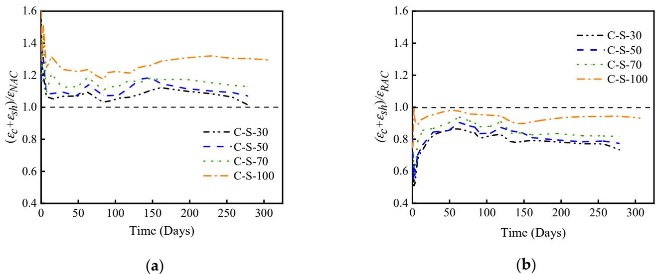
**Figure 7.** Comparing the deformation of SRAC with two control groups. (a) Comparing the deformation of SRAC and NAC. (b) Comparing the deformation of SRAC and RAC.
