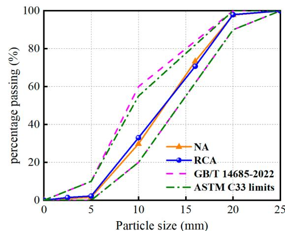
**Figure 2.** Gradation curve for coarse aggregate.
