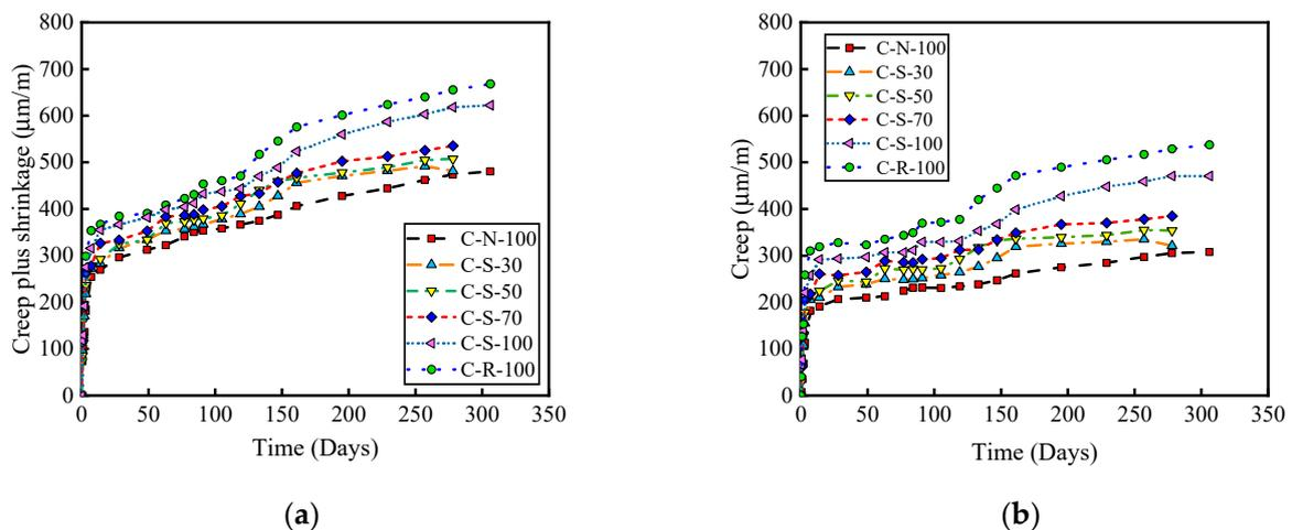
**Figure 5.** The curve of creep and shrinkage deformation over time. (a) Creep plus shrinkage. (b) Creep.
