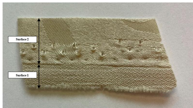
**Figure 4.** Fragment of waste textile material (green PES). Polyester waste material, before shredding, used to make the packing elements.
