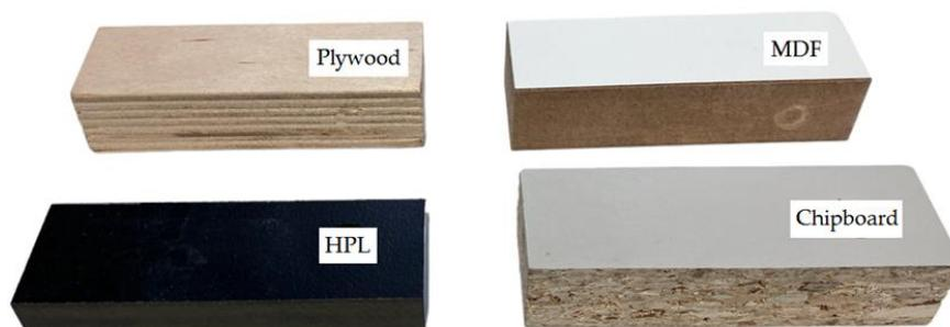
Figure 1. The test materials.
