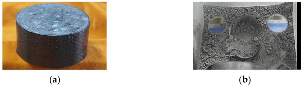
**Figure 2.** Failure mode of concrete specimen: (a) pre-failure specimen; (b) post-failure specimen.
