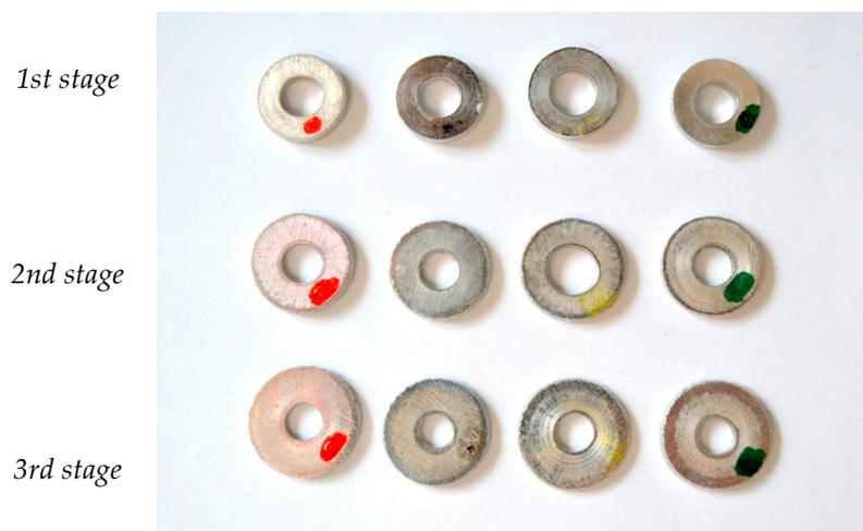
**Figure 7.** Rings after each compression stage using four lubricants. From left to right: copper paste, silicone oil, MoS<sub>2</sub> grease, aluminum anti-size.
