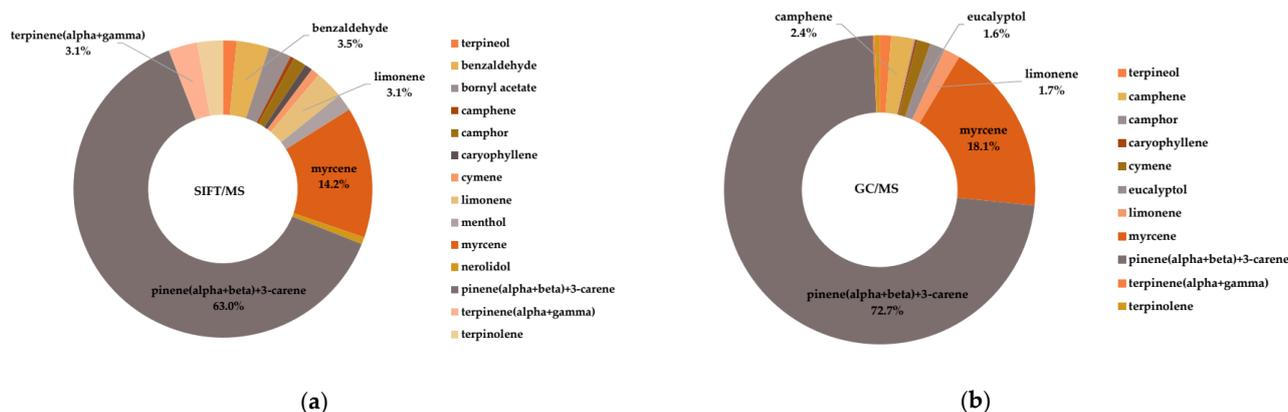
**Figure 6.** Detailed components of NVOC concentration. (a) Percentage of detailed components of NVOC emissions recorded through SIFT-MS analysis; (b) Percentage of detailed components of NVOC emissions recorded through GC-MS analysis.
