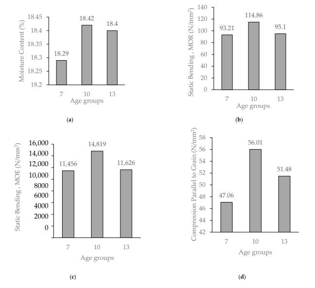
**Figure 9.** (a) Moisture content; (b) static bending, MOR; (c) static bending, MOE; (d) compression parallel to grain results of untreated *Acacia mangium* superbulk [22].
