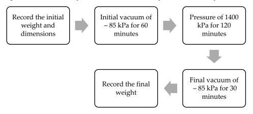
Figure 7. The flowchart for the treatment process.
