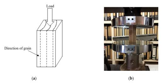
**Figure 4.** (a) The compression parallel to the grain test [13]; (b) the compression parallel to the grain test at the laboratory.
