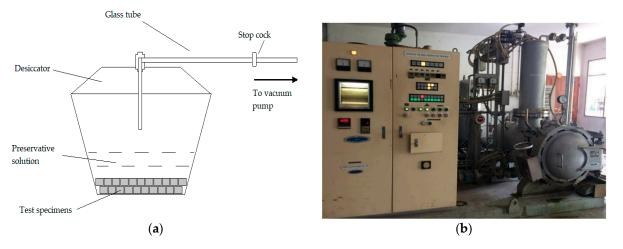
Figure 6. (a) The treatability test vacuum desiccators setup [13]; (b) treatment process machine.
