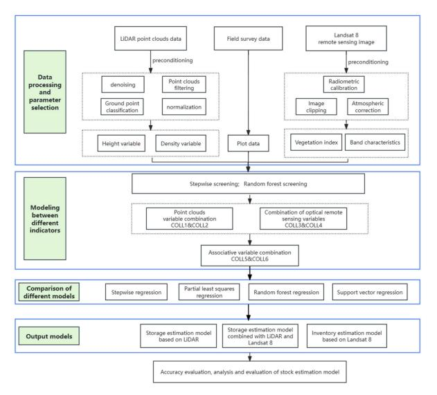
and support vector regression were used to construct the model, and the accuracy of the model was analyzed and evaluated by combining the field investigation data.
