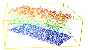
**Figure A1.** Cloud processing results of sample locations. The height increases from blue to red, with blue representing the ground and red representing the forest canopy.
