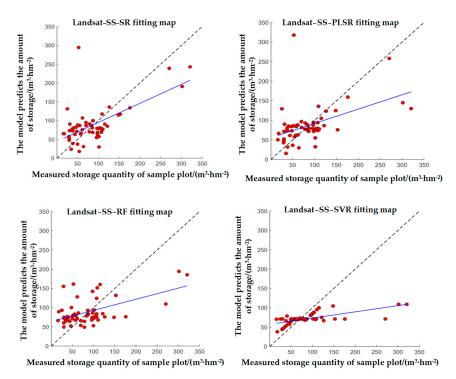
**Figure 5.** Optical remote sensing data volume estimation model fitting based on stepwise selection method.
