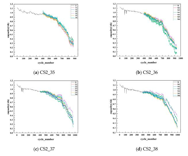
**Figure 13.** Multiple model comparison experiments of CALCE battery (400 predicted starting points). (a) Comparative experiment for battery CS2\_35; (b) comparative experiment for battery CS2\_36; (c) comparative experiment for battery CS2\_37; and (d) comparative experiment for battery CS2\_38.
