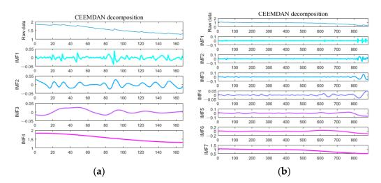
**Figure 9.** CEEMDAN decomposition of battery capacity data. (a) Decomposition of B0005; (b) decomposition of CS2\_35.
