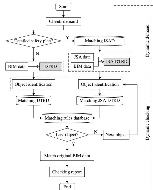
Figure 11. Algorithm of dynamic safety checking.
