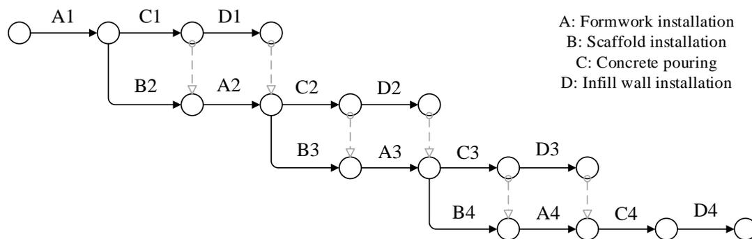
**Figure 12.** Overall construction PERT of the building (The number indicates which layer it is).
