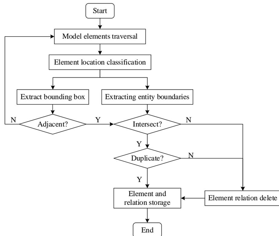
Figure 6. Entities' relationship extraction process in BIM model.
