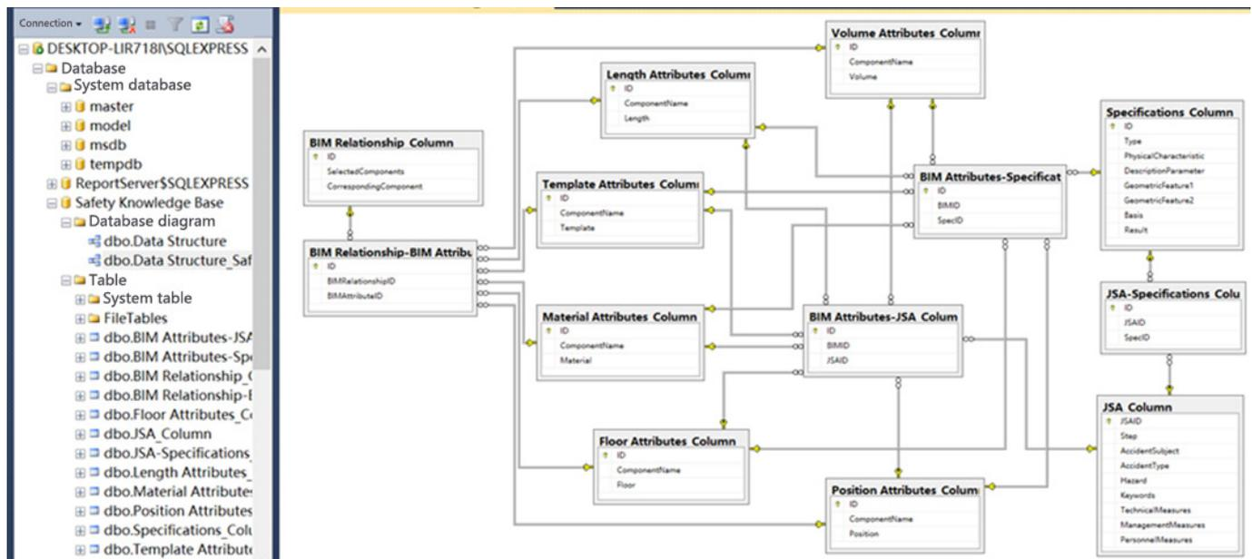
Figure 3. Knowledge base integrating both safety rules and topological BIM elements.
