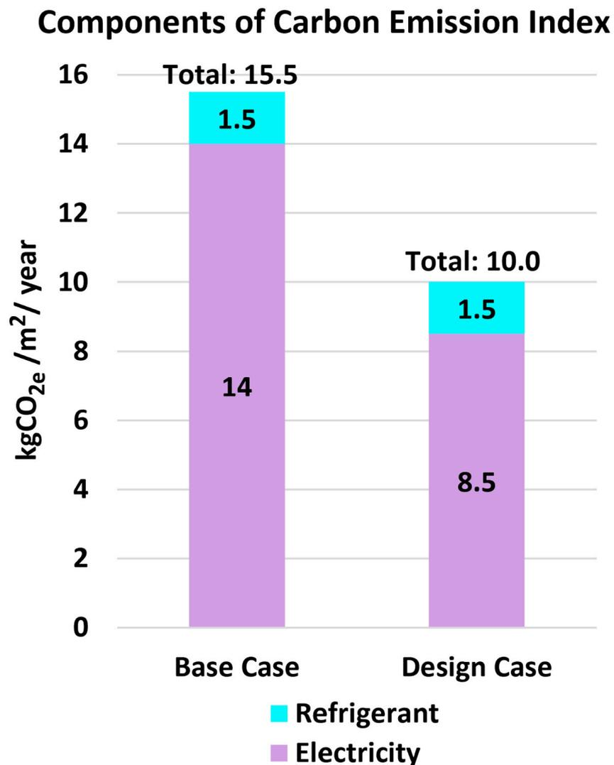
**Figure 5.** Carbon emission index (CEI) and its components for the conventional building (base case) and the Zero Carbon Ready green building (design case).
