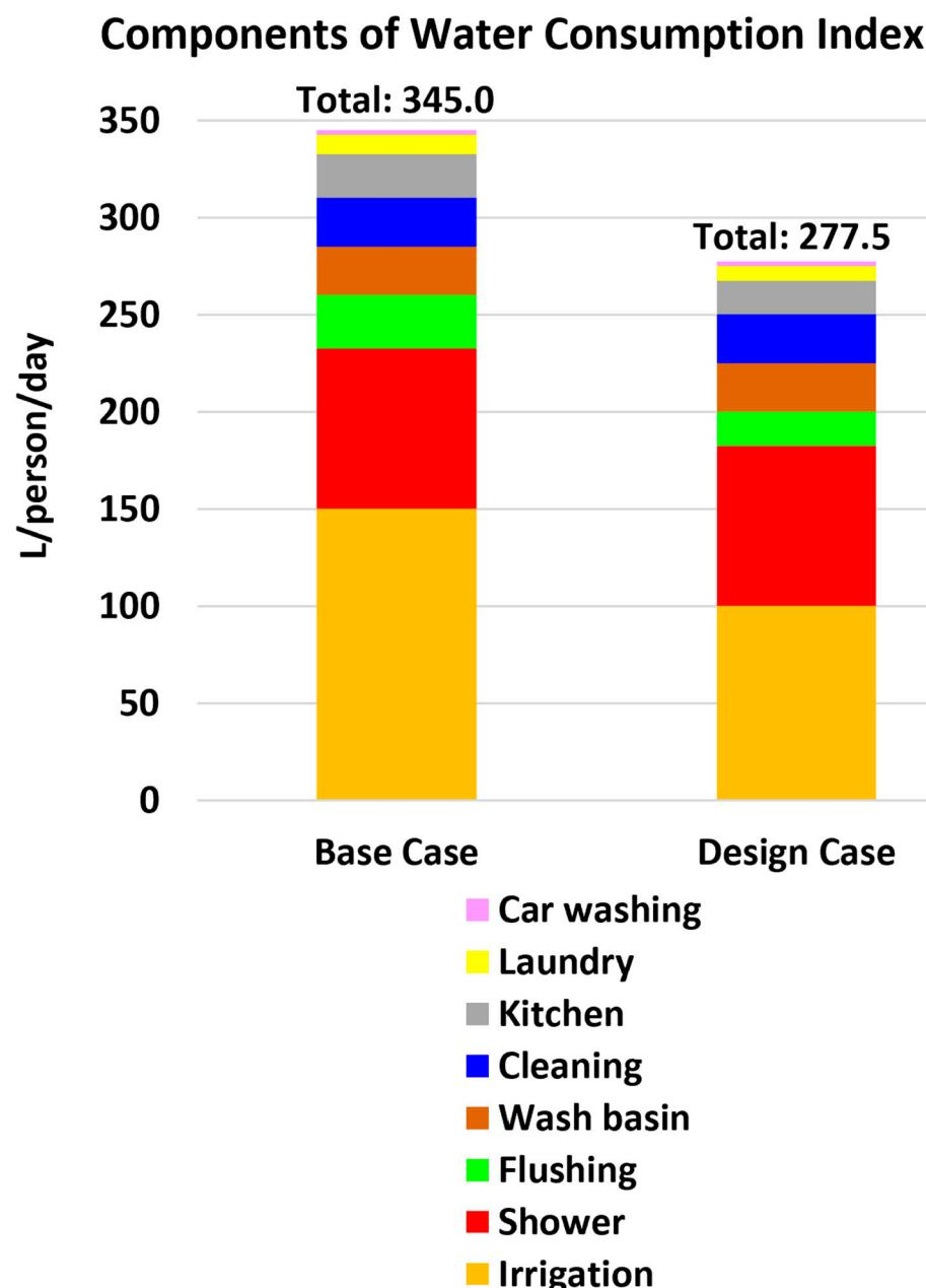
**Figure 7.** Water consumption index (WCI) and its components for the conventional building (base case) and the Zero Carbon Ready green building (design case).
