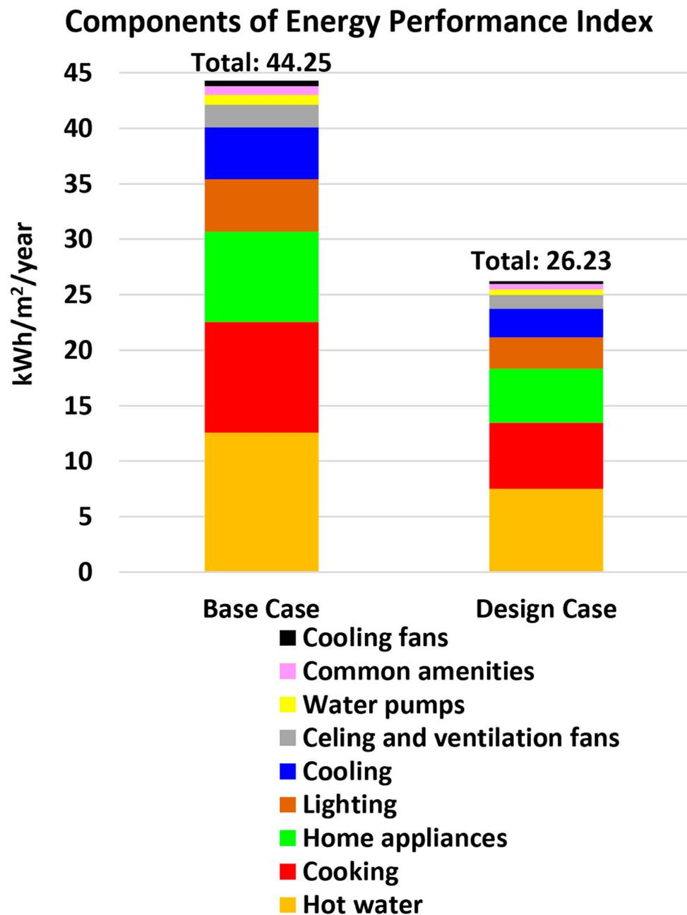
**Figure 6.** Energy performance index (EPI) and its components for the conventional building (base case) and the Zero Carbon Ready green building (design case).
