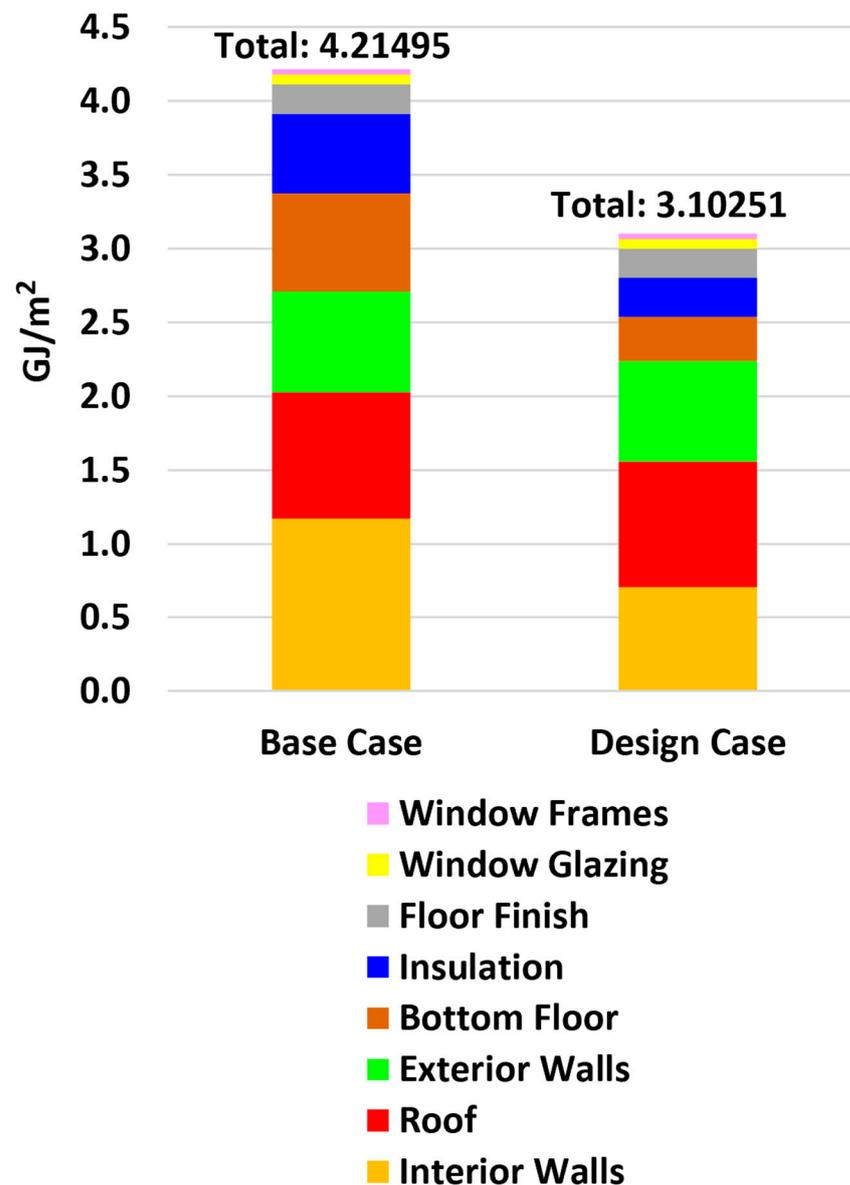
**Figure 8.** Embodied Energy Index (EEI) and its components for the conventional building (base case) and the Zero Carbon Ready green building (design case).
