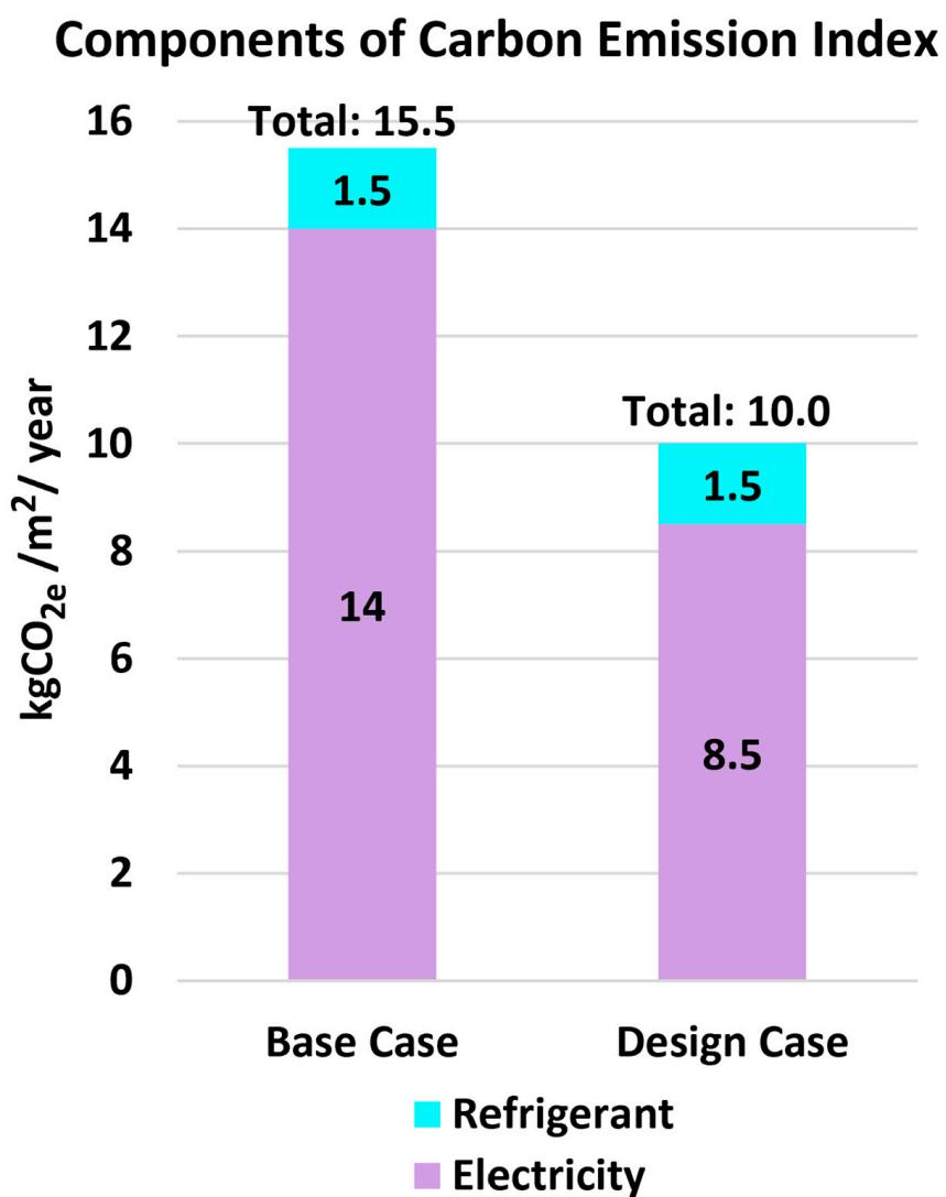
**Figure 5.** Carbon emission index (CEI) and its components for the conventional building (base case) and the Zero Carbon Ready green building (design case).
