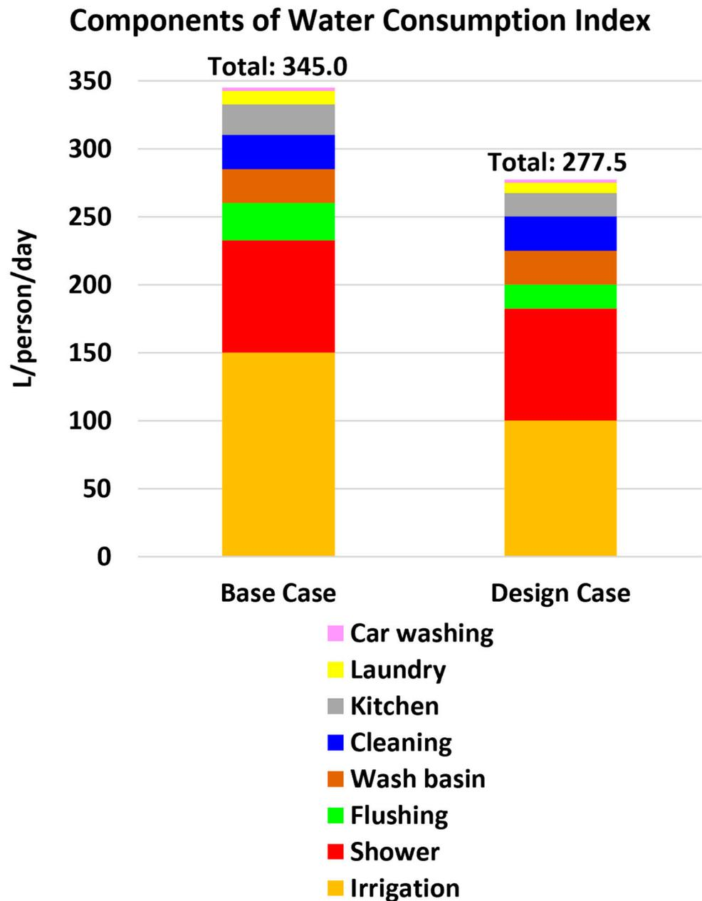
**Figure 7.** Water consumption index (WCI) and its components for the conventional building (base case) and the Zero Carbon Ready green building (design case).
