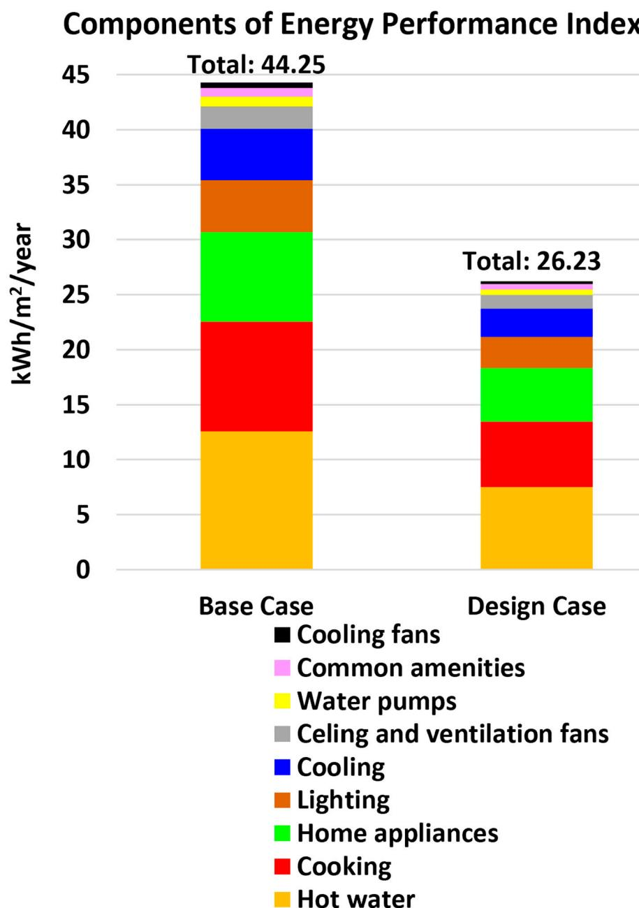
**Figure 6.** Energy performance index (EPI) and its components for the conventional building (base case) and the Zero Carbon Ready green building (design case).
