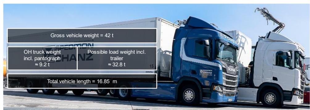
**Figure 2.** Visualization of OH trucks with extended and lowered pantographs.
