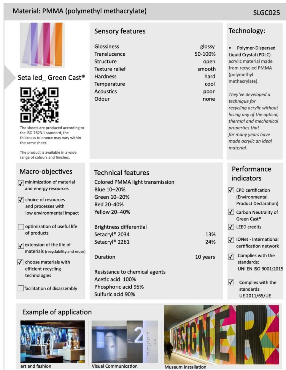
**Figure 4.** Example of standard sheet. Performance indicators refer to the technical standards provided by the producers [54–56].
