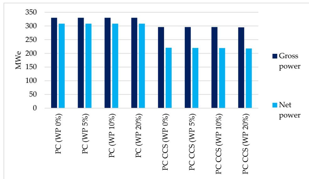
**Figure 4.** Graph of PC gross power and net power output without and with retrofitting of CCS technology.
