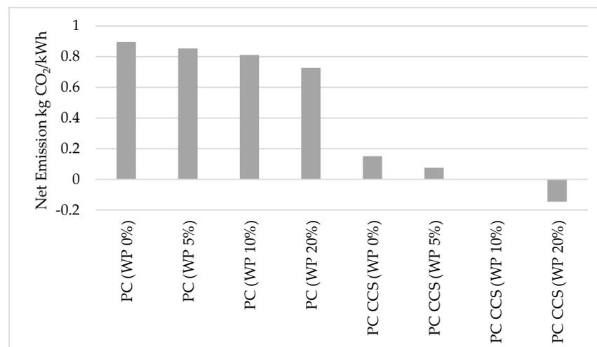
**Figure 6.** Net emissions of CO<sub>2</sub> without and with CCS retrofitting of PC.
