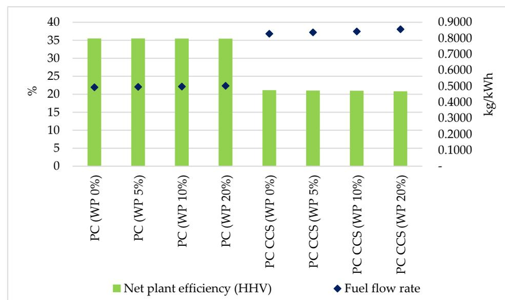
**Figure 5.** Graph of PC efficiency and fuel flow rate without and with retrofitting of CCS technology.
