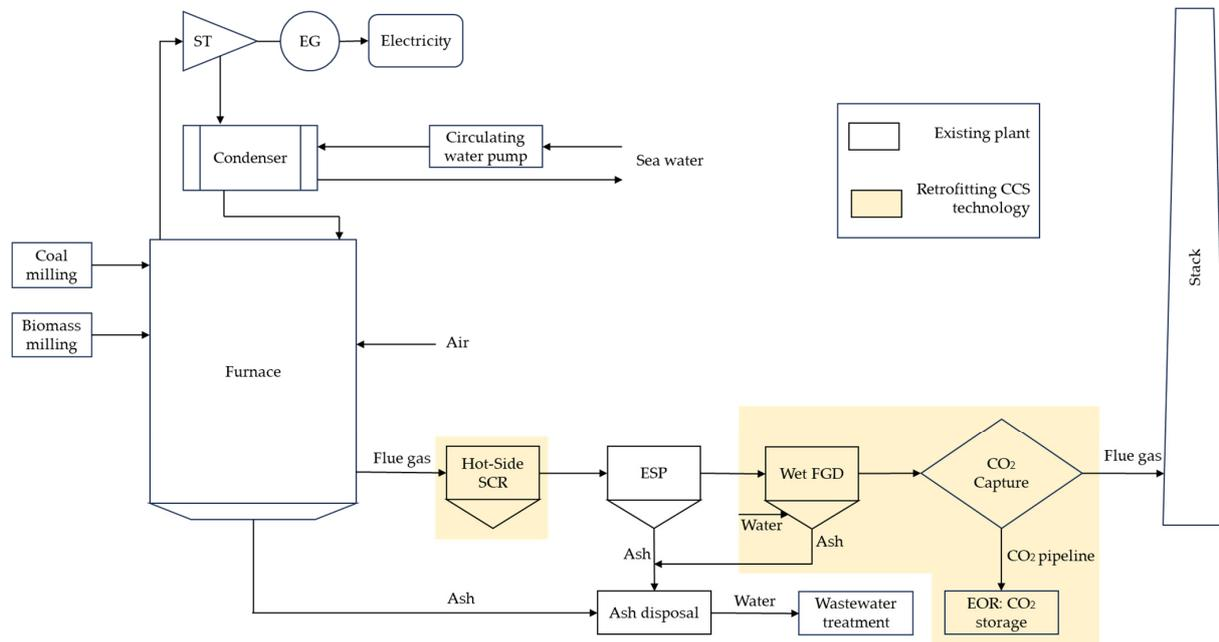
**Figure 3.** Diagram of the Indramayu CFPPs with existing and retrofitting technology (SCR, FGD, and CCS).
