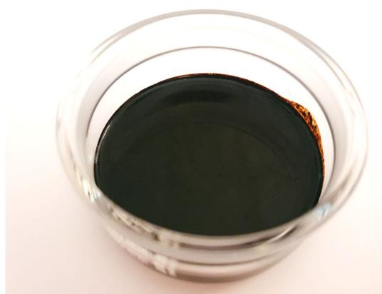
**Figure 6.** Bio-oil produced from black liquor pyrolysis–BL<sub>PYOIL</sub>.
