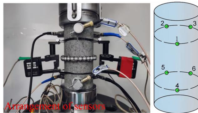
**Figure 3.** Acoustic emission monitoring system.
