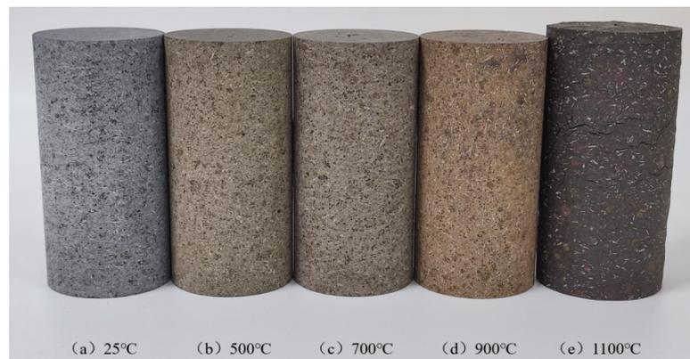
**Figure 4.** Basalt apparent morphology.
