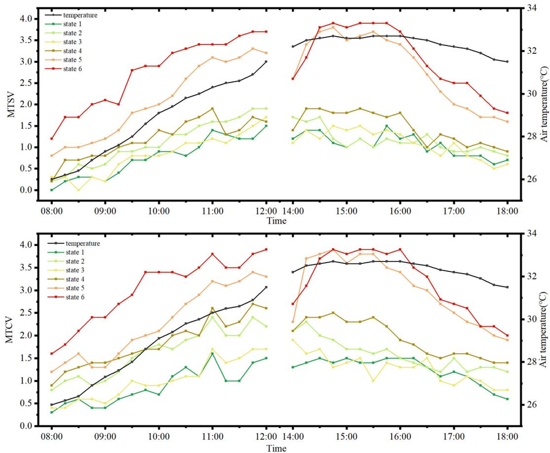
**Figure 5.** Thermal sensation and thermal comfort votes of personnel over time under different states.
