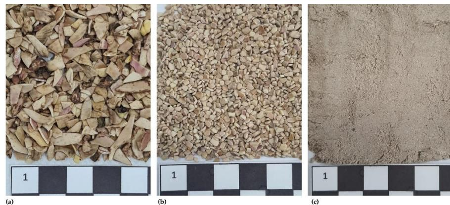
**Figure 2.** Pistachio shell grain sizes: (a) Pg shells with dimensions ranging from 2 to 4 mm; (b) Pf shells with dimensions of 0.5–2 mm; (c) Ps shells with dimensions <0.5 mm. Figures report the metric reference to 1 cm.
