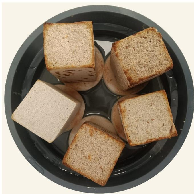
**Figure 6.** Water absorption test by capillarity.
