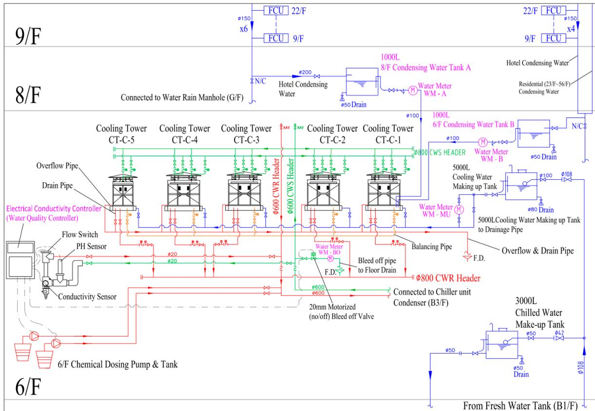
**Figure 5.** Schematic for reclaiming condensed water system.
