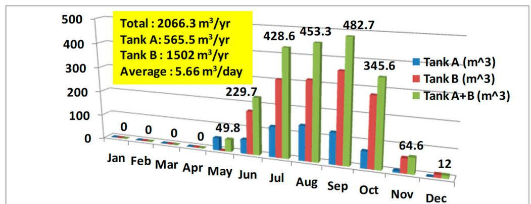
Figure 8. Reclaimed condensed water records.
