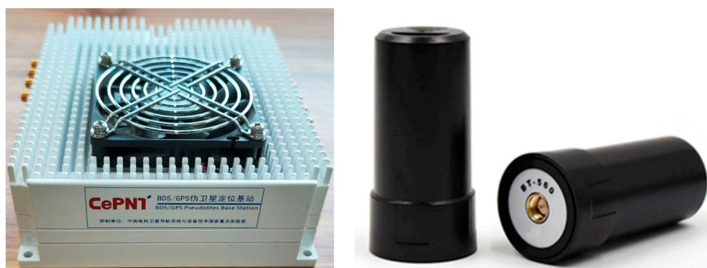
**Figure 1.** Eight-channel indoor array pseudo-satellite base station and transmitting antenna.
