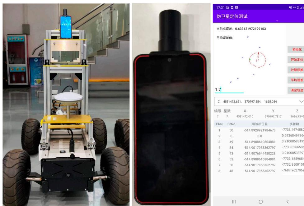
**Figure 7.** Unmanned robot platform and indoor pseudo-satellite receiver data acquisition equipment based on high-gain antennas.
