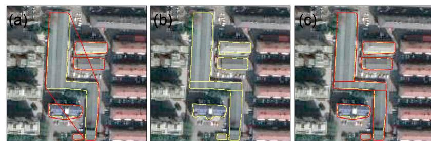
**Figure 3.** The figure shows how the building is divided. Yellow indicates the outline of the original building, and red indicates the convex hull. (a) represents the convex hull before segmentation of the building contour. (b) represents the building contour after segmentation. (c) represents the convex hull after segmentation of the building contour.
