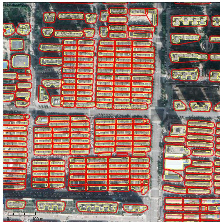
**Figure 10.** The figure shows the adaptive buffer results. The yellow polygon area represents the building contours, and the red polygon represents the adaptive buffer.
