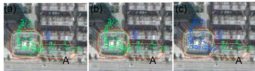
**Figure 6.** The figure shows repeat point detection and deletion. The yellow polygon represents the building contour, and the red polygon represents the adaptive buffer. (a) Original point data (shown in green); (b) supplementary selection results of building A (green); (c) repeat point detection and deleting results of building A (green); blue represents the rest of the original point data.
