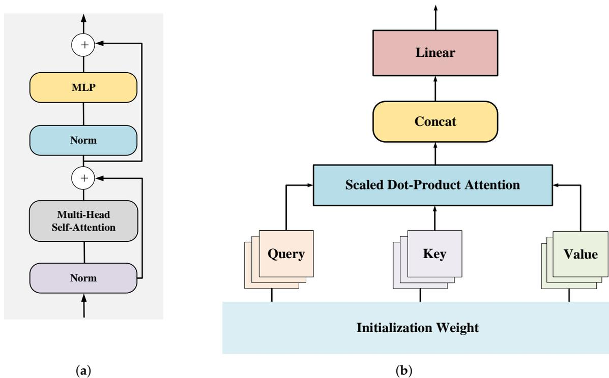
**Figure 4.** Graphical representation of the transformer encoder: (a) The general structure of encoder blocks. (b) Multi-head self-attention mechanism.
