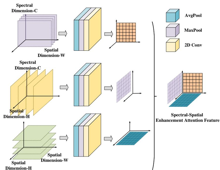
**Figure 3.** Illustration of SSEA. It consists of three branches that establish the dependencies between the spectral dimension  $C$  and the spatial dimensions  $H$  and  $W$  by means of rotational operations, and it computes the attention weights in each of the three directions.
