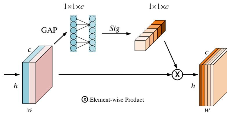
**Figure 2.** Illustration of ECA. It uses global average pooling and a one-dimensional convolution operation with an adaptive convolution kernel to compute the weights under each band, followed by an activation function to implement the mapping of the attention weights.
