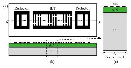
**Figure 2.** Schematic of the top view (**a**), the cross-sectional view at (A-B) (**b**), and the modeling periodic cell (**c**) of the one-port SAW resonator.
