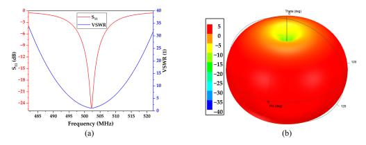
**Figure 9.** (a) Simulated  $S_{11}$  and VSWR of helix antenna; (b) the normalized radiation pattern of the antenna.
