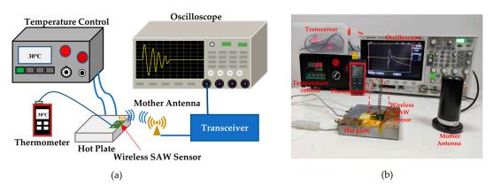
**Figure 5.** (a) Schematic diagram of the wireless temperature test platform; (b) self-built temperature test platform.
