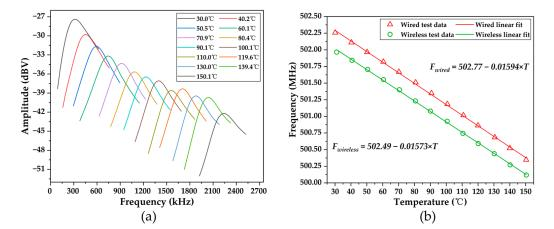
**Figure 12.** (**a**) Echo signal in the frequency domain at different temperatures; (**b**) comparison of the frequency and temperature relationship between the wired test and wireless test.
