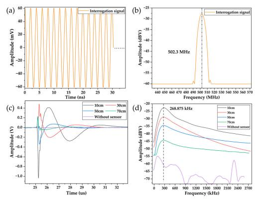
**Figure 11.** (**a**) Interrogation signal in the time domain; (**b**) interrogation signal in the frequency domain; (**c**) echo signal at different distances in the time domain; and (**d**) echo signal at different distances in the frequency domain.
