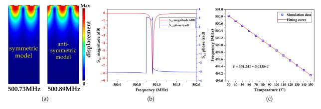
**Figure 6.** Simulation results of SAW resonator: (a) Rayleigh symmetry mode and anti-symmetry mode; (b) magnitude and phase of return loss  $S_{11}$ ; and (c) variation in the resonant frequency with temperature.
