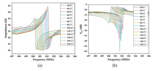
**Figure 10.** Impedance curve (**a**) and return loss  $S_{11}$  curve (**b**) of the SAW sensor at different temperatures after matching.
