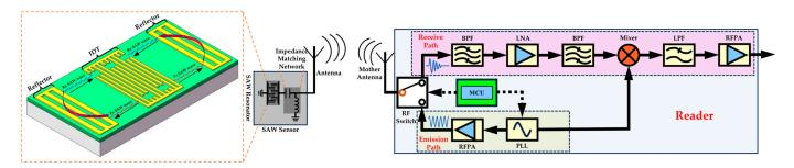
Figure 1. Schematic diagram of the constructed wireless temperature measurement system.
