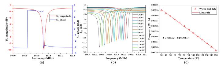
**Figure 8.** Wired measured results of the SAW resonator (**a**) magnitude and phase of return loss  $S_{11}$ ; (**b**) the  $S_{11}$  curve at different temperatures; and (**c**) the frequency of the SAW resonator as a function of temperature.
