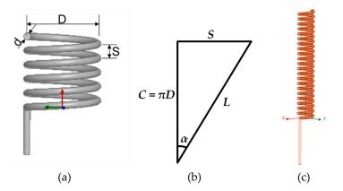
**Figure 4.** (a) Schematic diagram of the helix antenna; (b) relationship between space (*S*), helix diameter (*D*), angle of lift ( $\alpha$ ), and circle length (*L*); and (c) modeled helix antenna in HFSS.
