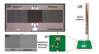
**Figure 7.** (a) Micro-view of the designed SAW resonator; (b) micro-view of the IDT and reflector; (c) view of the SAW sensor with impedance matching network; and (d) view of the wireless SAW temperature sensor.
