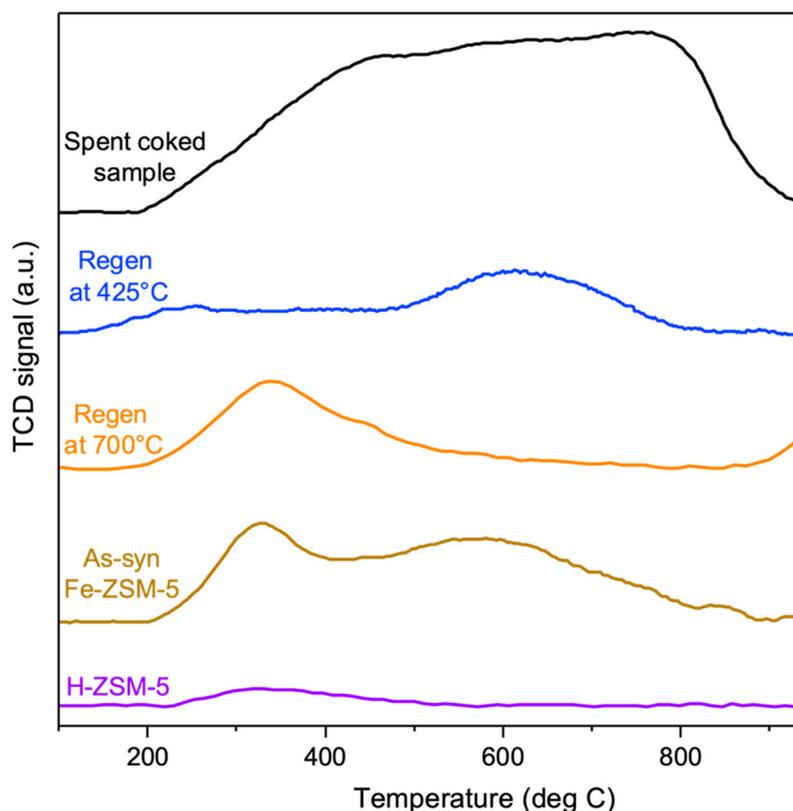
**Figure 7.** H<sub>2</sub> TPR analysis of H-ZSM-5 (shown in purple); isomorphous substituted as-synthesized Fe-ZSM-5 (shown in brown); fully regenerated, coke-free catalyst (created by removing both soft and hard coke by oxidative treatment at 700 °C, shown in orange); catalyst containing only hard coke (created by removing soft coke by oxidative treatment at 425 °C, shown in blue); and fully spent, coked sample (deactivated for 14 h in MDA at 700 °C, shown in black).
