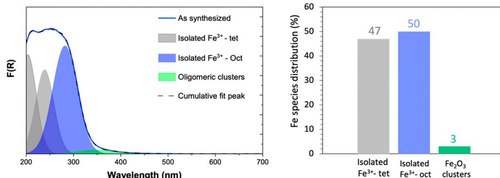
**Figure 3.** UV-Vis analysis on isomorphous as-synthesized Fe-ZSM-5 catalyst to determine Fe species distribution.
