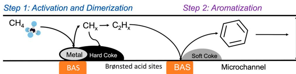
**Figure 8.** Schematic illustrating the formation of different types of coke (soft versus hard coke) on active sites.
