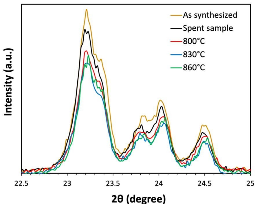
**Figure 11.** X-ray diffraction (XRD) analysis was conducted on the as-synthesized sample, spent sample, and spent sample thermally treated at temperatures ranging from 800 °C to 860 °C for 30 min in 0.5 SCCM of Ar flow.
