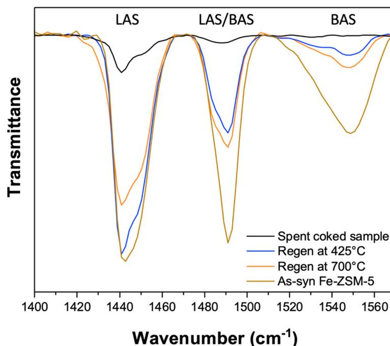
**Figure 6.** Pyridine FTIR analysis of as-synthesized Fe-ZSM-5 catalyst (shown in brown); fully regenerated, coke-free catalyst (created via oxidative treatment at 700 °C, shown in orange); catalyst containing only hard coke (created via oxidative treatment at 425 °C, shown in blue); and fully spent, coked sample (deactivated for 14 h in MDA at 700 °C, shown in black).
