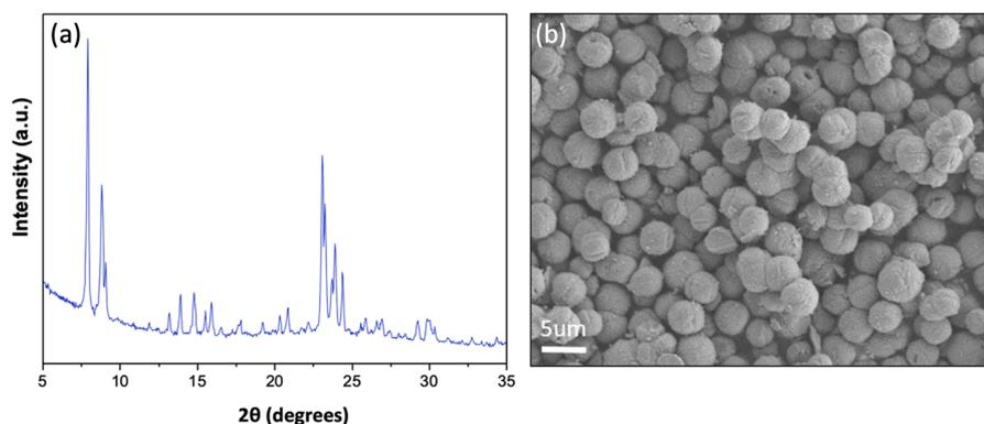
**Figure 2.** (a) X-ray diffraction analysis of Fe-ZSM-5 showing MFI peaks. (b) Scanning electron microscope image of synthesized Fe-ZSM-5. Synthesis conditions for pure Fe-ZSM-5 (molar ratios): Si/Fe = 46.1, Si/Al = 40, TPAOH/TEOS = 0.1, NaOH/TEOS = 0.2, H<sub>2</sub>O/TEOS = 40.45, temperature = 175 °C.
