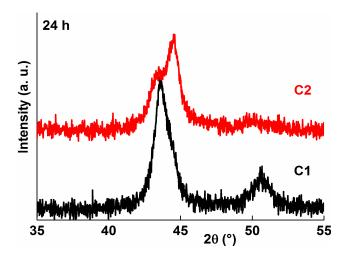
Figure 1. XRD patterns in the 20 range of (35–55)° of the milled C1 and C2 powders for 24 h.
