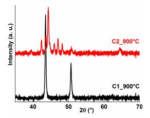
Figure 4. XRD patterns of the heat-treated C1 and C2 powders in the DSC.
