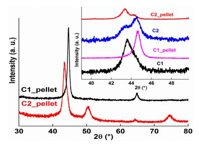
**Figure 2.** XRD patterns of the sintered C1\_pellet and C2 pellet for 1 h at 500 °C. The inset shows the comparison of the main diffraction peak of the powders and pellets.
