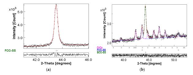
**Figure 5.** Rietveld refinement of the XRD patterns of the C1\_900 °C and C2\_900 °C samples taken in the 2-theta range of (35–55)° for: (**a**) C1\_900 °C alloy; and (**b**) C2\_900 °C alloy.
