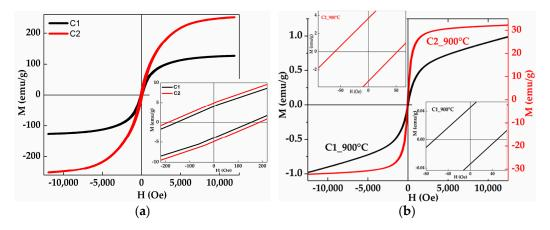
**Figure 7.** (a) Hysteresis loops of the mechanically alloyed C1 and C2 for 24 h; (b) C1\_900 °C and C2\_900 °C. Insets show the enlargement of the central parts.
