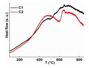
Figure 3. DSC curves of the ball-milled C1 and C2 powders for 24 h.
