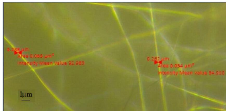
**Figure 2.** PMMA nanofibers net deposited at 15 kV.
