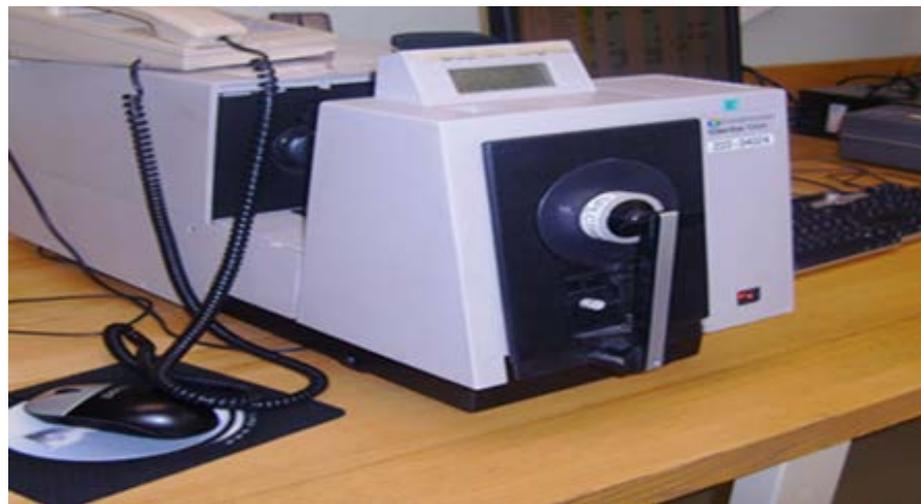
**Figure 2.** X-rite-7000A spectrophotometer.
