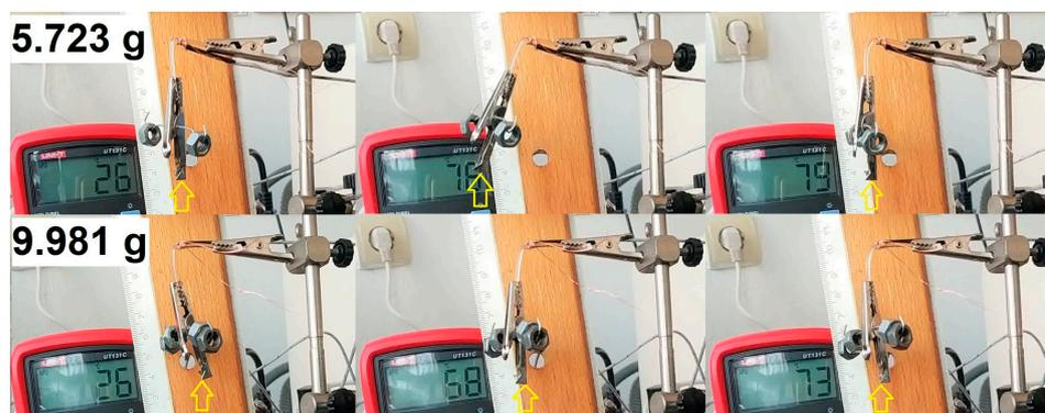
**Figure 6.** Recorded images illustrating the development of work-generating SME during the heating of R-PETG filaments with two different applied loads.
