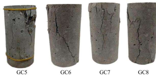
**Figure 6.** Failure patterns of each group of specimens with 40% coal gangue content.
