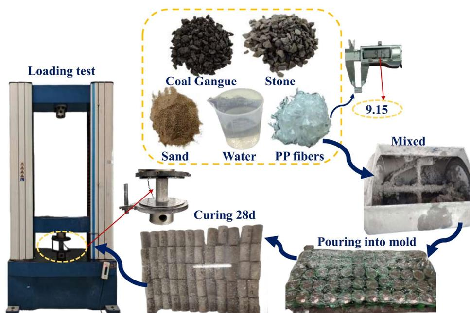
**Figure 1.** Concrete preparation process.
