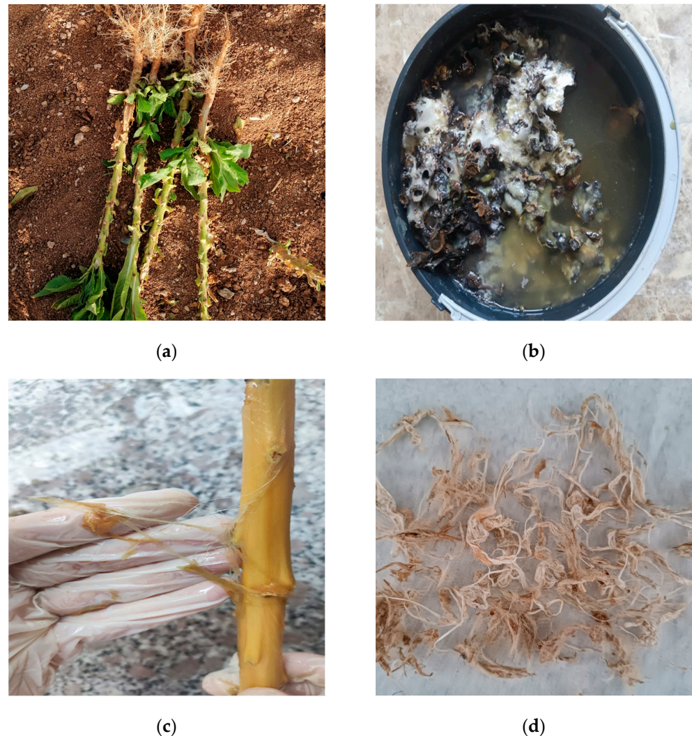
Figure 1. Fiber extraction from NRL plant stalk waste. (a) Waste NRL plant stalks, (b) NRL plant stalks retting in water, (c) fibers removed from stalks and washed with distilled water, and (d) extracted dry NRL fibers.
