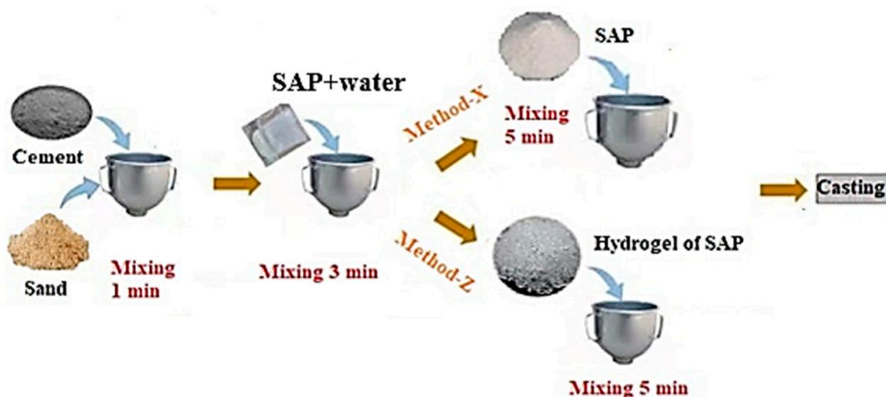
**Figure 3.** The systematic procedure of preparing cement mortars modified with SAPs derived from Method-X and Method-Z.
