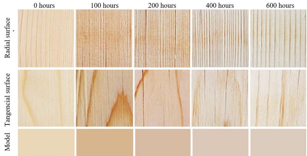
**Figure 5.** Color variation in spruce wood specimens during accelerated aging (wet mode).
