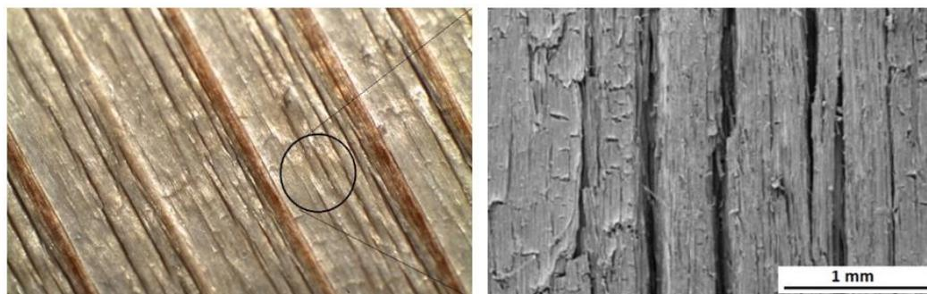
**Figure 12.** Morphology of radial spruce wood surface after 600 accelerated aging hours (wet mode).
