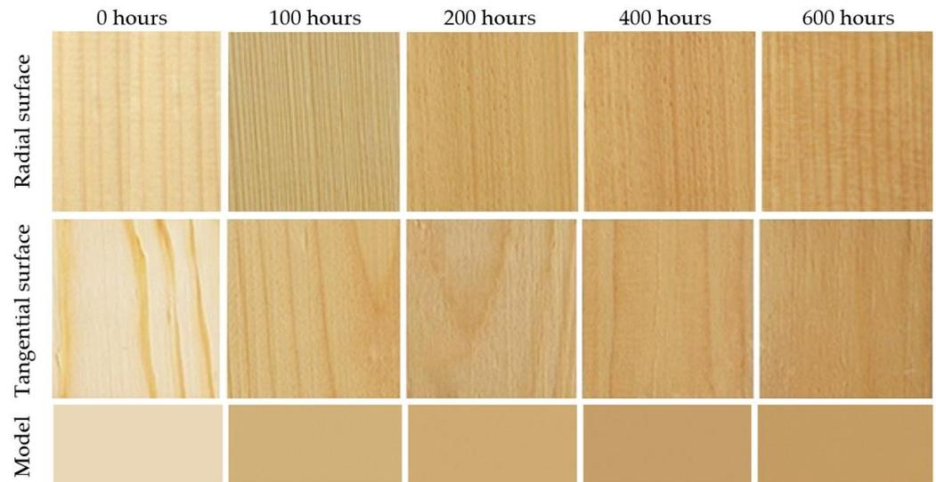
**Figure 3.** Color variation in spruce wood specimens during accelerated aging (dry mode).
